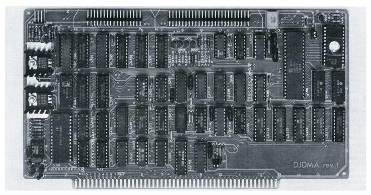
The DISK JOCKEY® DMA FLOPPY DISK CONTROLLER (DJ/DMA) is an IEEE 696 (S-100) compatible floppy disk controller which contains logic to implement Direct Memory Access (DMA) operations on the
