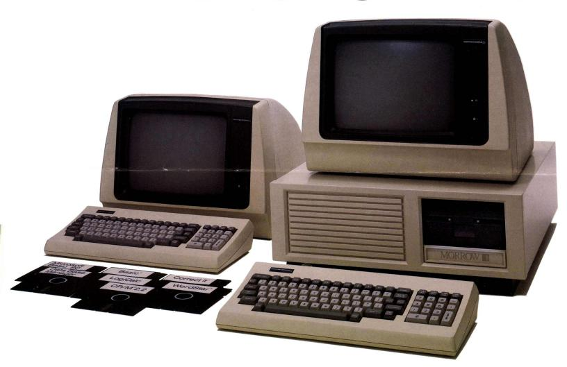
The Decision 1 is a flexible microcomputer that can be configured as a single user system running CP/M, or can be expanded to a sophisticated multi-user system running the Micronix Operating System.
