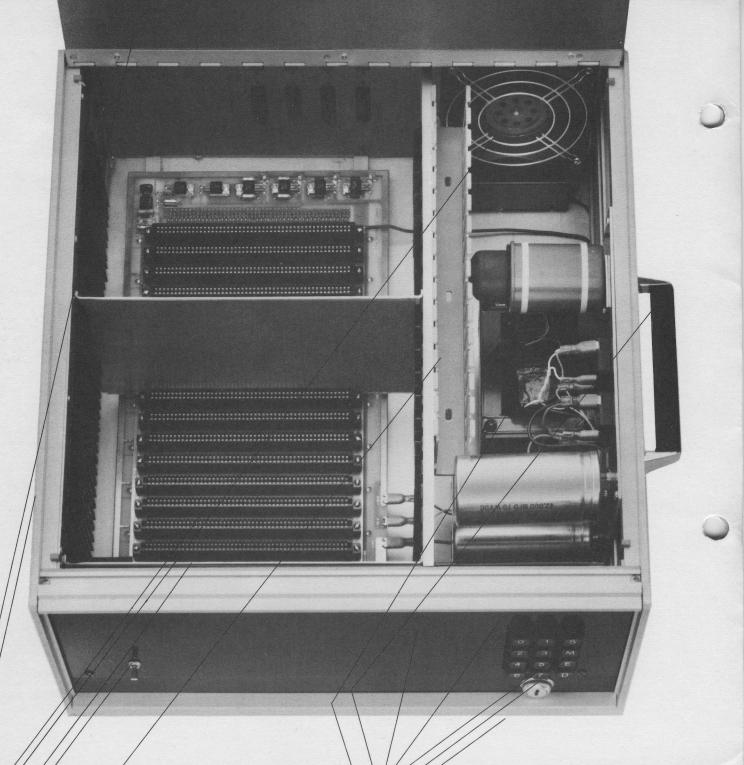
**WIRING CHANNEL\***, cord wrap\* and detachable line cord help keep your system neat.
