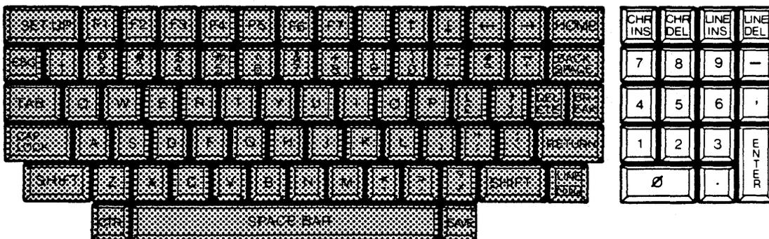
Fig. 2-6: Morrow Designs Terminal - Numeric Keyboard
