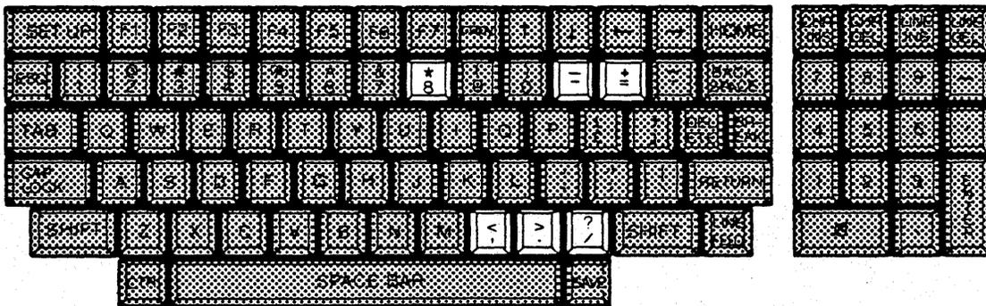
Fig. 2-7: Morrow Designs Terminal - Special Symbol Keys
