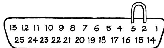
Figure 2: Jumpering DTE connector pins 2 and 3.
