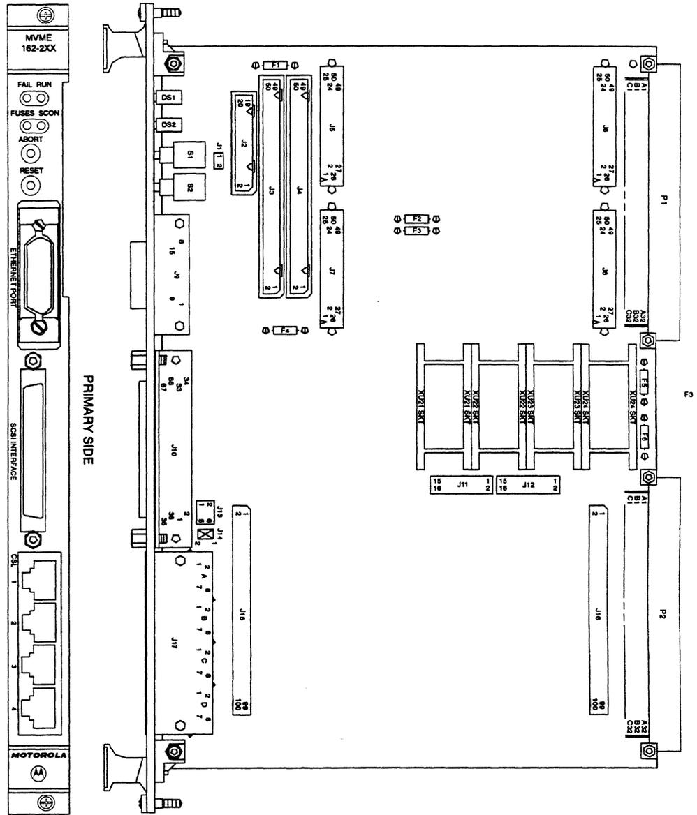
MVME162LX Switch, Header, Connector, Fuse, and LED Locations
