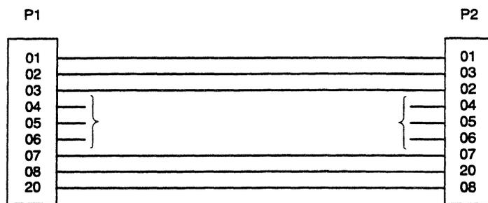
Figure 3. CENTRONICS Parallel Cable Connections for MVME338
