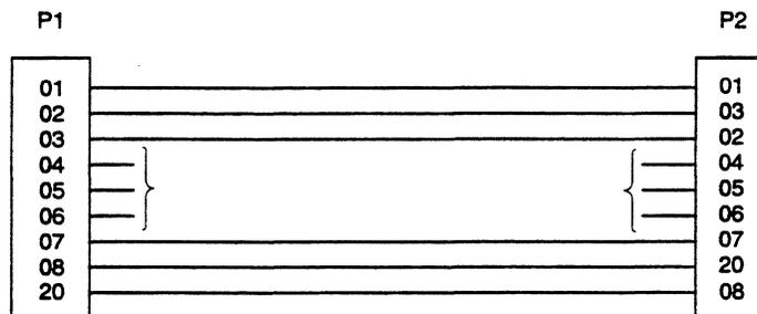
Figure 3. EIA-232-D Terminal/Printer Cable Connections
