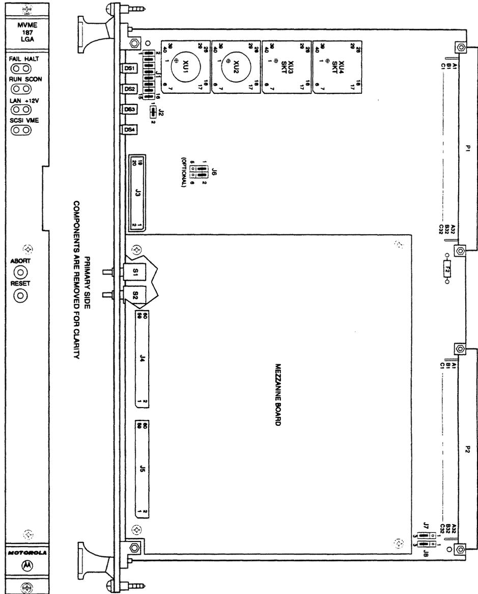
MVME187 Switch, Header, Connector, Fuse, and LED Locations
