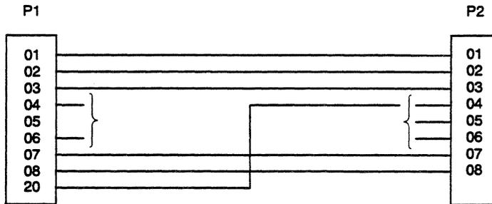
**Figure 2. EIA-232-D Remote Printer Cable Connections**
