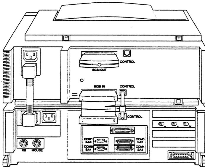
**Rear View of System with SCSI Module Installed**
