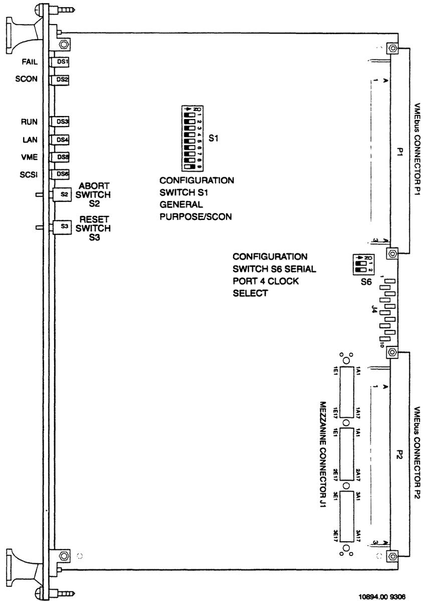
MVME197DP / SP Switch, Header, Connector, Fuse and LED Locations
