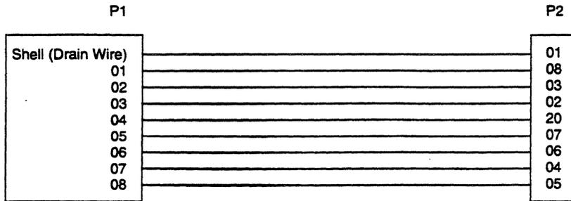
**Figure 4. EIA-232-D DB9-to-DB25 Serial Adapter Cable Connections**
