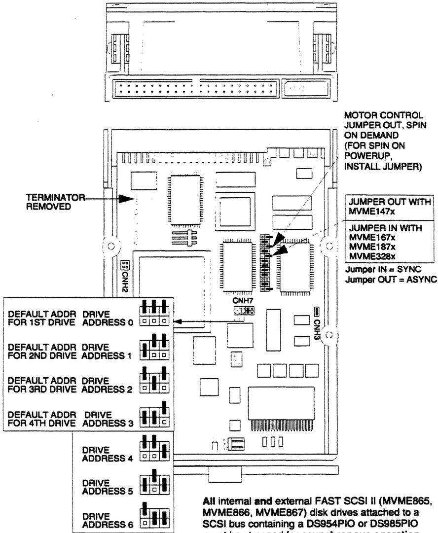
All internal and external FAST SCSI II (MVME865, MVME866, MVME867) disk drives attached to a SCSI bus containing a DS954PIO or DS985PIO must be strapped for asynchronous operation, regardless of their associated SCSI controller.
