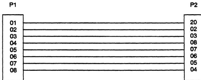
**Figure 5. EIA-232-D Straight-Through Cable Connections**
