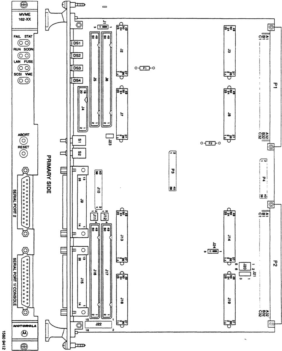
MVME162FX Switch, Header, Connector, Fuse, and LED Locations
