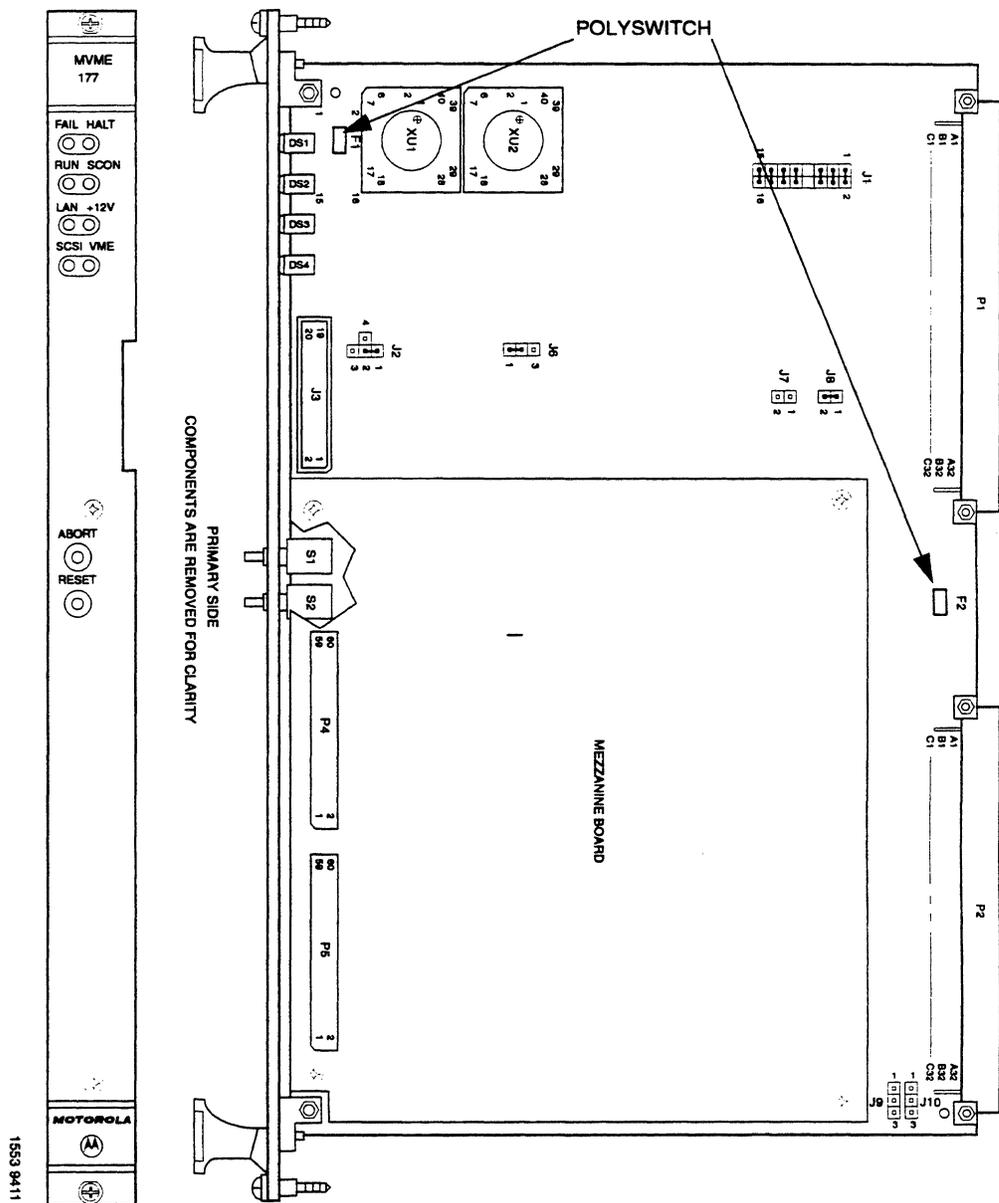
MVME177 Switch, Header, Connector, Polyswitch, and LED Locations
