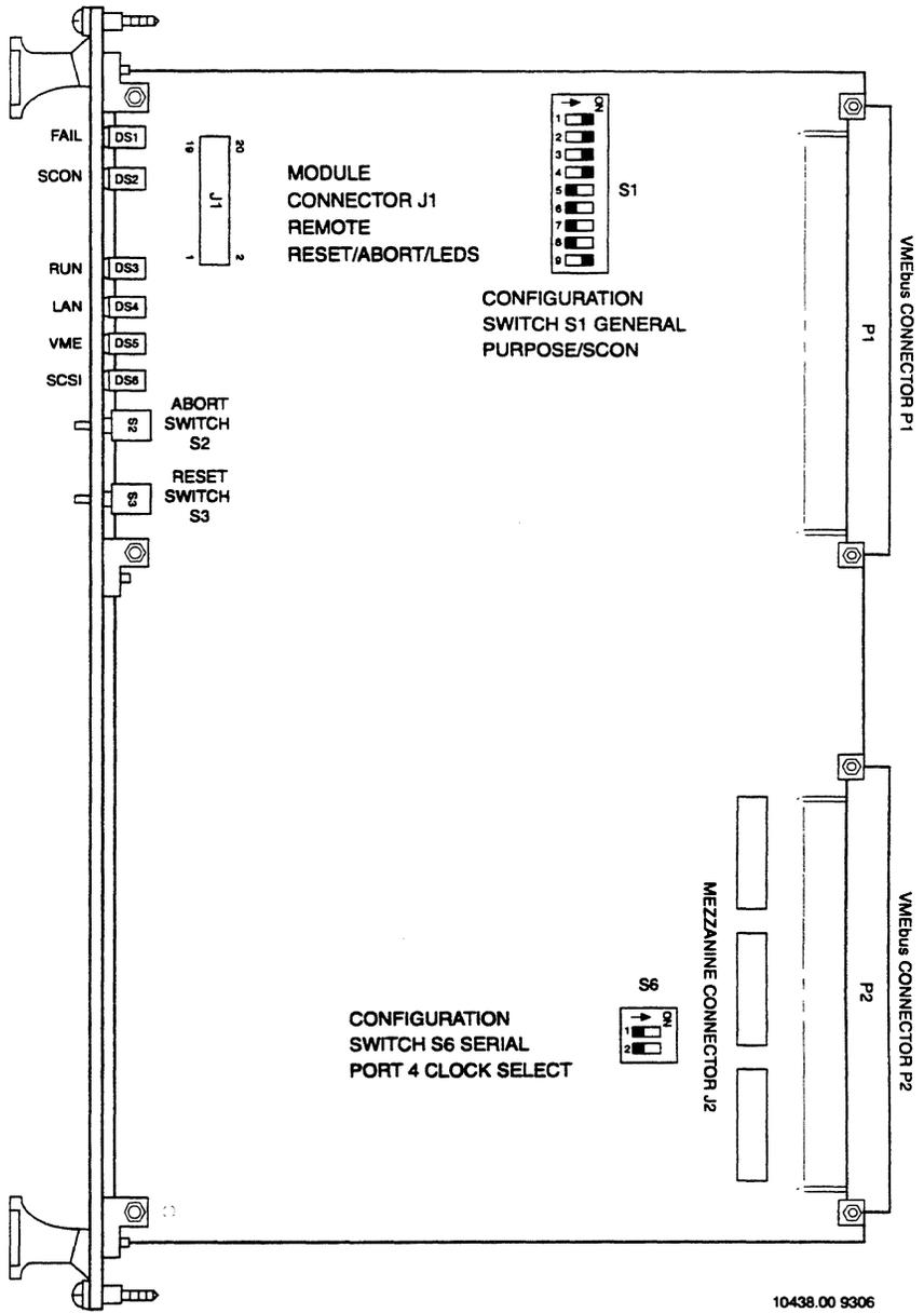
**MVME197LE Switch, Header, Connector, Fuse, and LED Locations**
