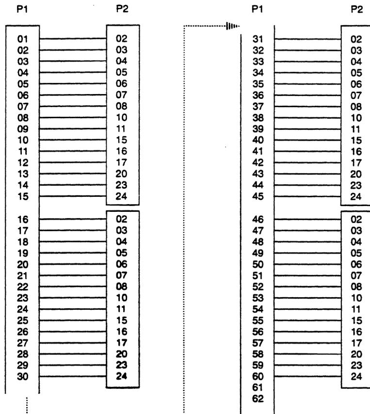
Figure 6. EIA-232-D HDA62-to-DB25 Quad Cluster Cable Connections
