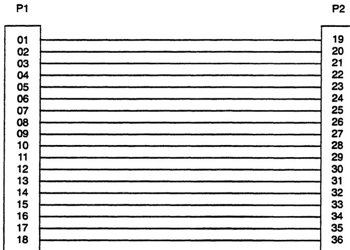
**Figure 1. CENTRONICS Parallel Straight-Through Cable Connections**
