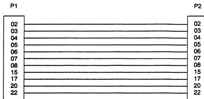
Figure 1. EIA-232-D Straight-Through Cable Connections
