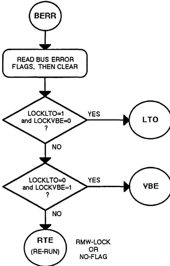
FIGURE 1. Bus Error Exception Handler Flowchart for MVME133XT
