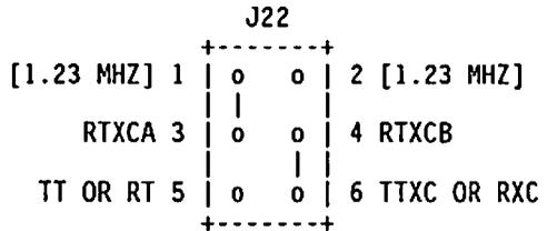
RTXCA IS DRIVEN BY ONBOARD 1.230769 MHZ. RTXCB IS DRIVEN BY TTXC IF PORT B IS CONFIGURED DCE (TO TERMINAL), OR FROM RXC IF PORT B IS CONFIGURED DTE (TO MODEM).
