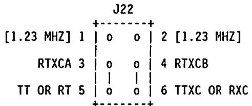
RTXCA IS DRIVEN BY TT+/- IF PORT A IS CONFIGURED AS A SLAVE, OR FROM RT+/- IF PORT A IS CONFIGURED AS A MASTER. RTXCB IS DRIVEN BY TTXC IF PORT B IS CONFIGURED DCE (TO TERMINAL), OR FROM RXC IF PORT B IS CONFIGURED DTE (TO MODEM).
