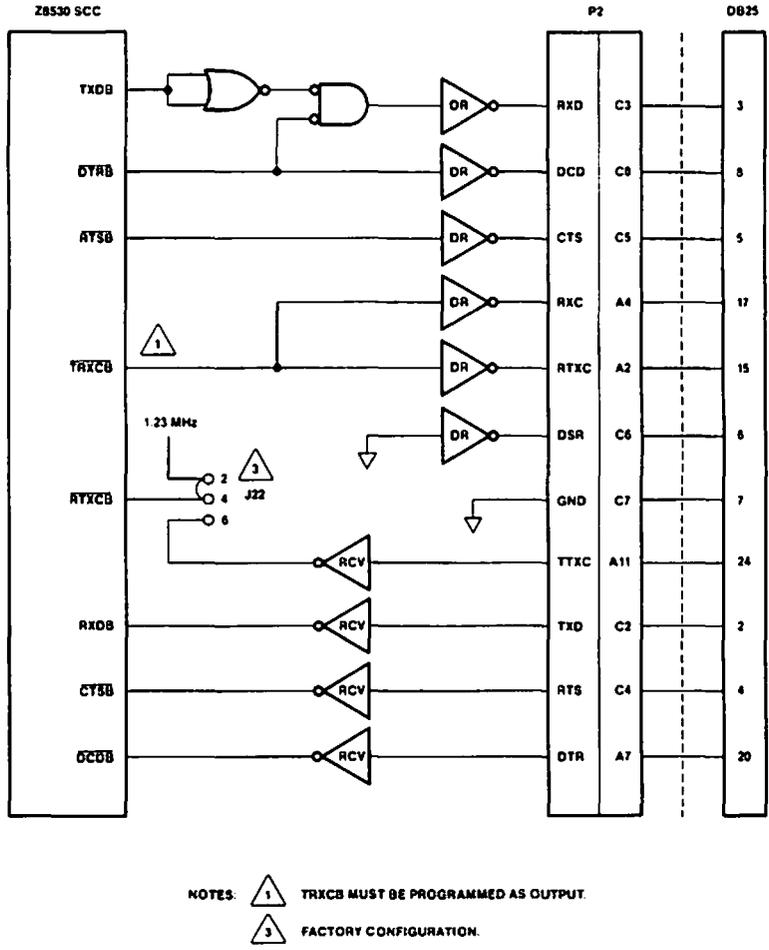
FIGURE 4-6. MVME133XT RS-232C Port Configured as DCE (To Terminal)
