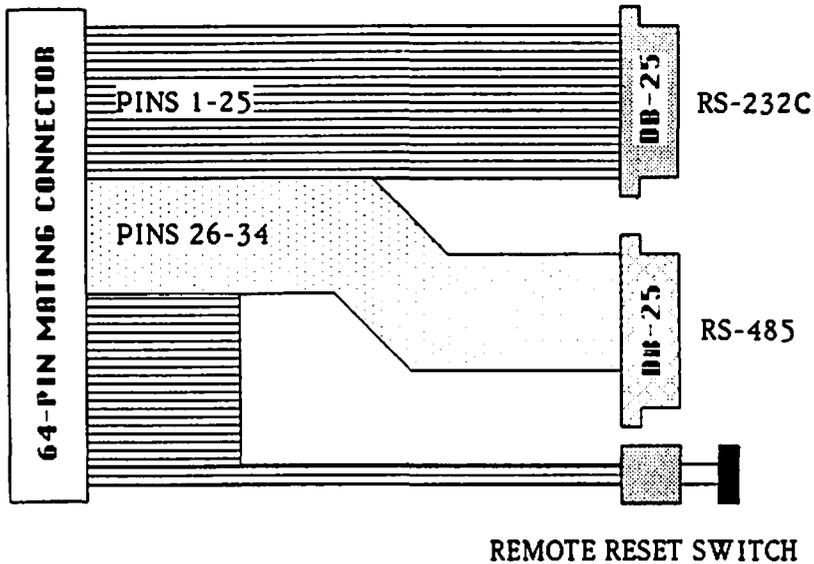
FIGURE 2-2. Cabling Connections to P2, Suggestion 1
