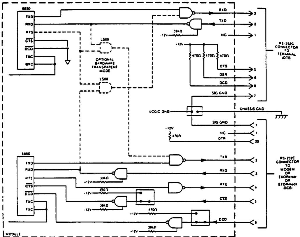
FIGURE 1. Middle-of-the-Road RS-232C Configuration
