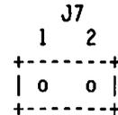
MVME133XT ONBOARD DRAM RESPONDS TO BOTH STANDARD (A24) ADDRESSING AND TO EXTENDED (A32) ADDRESSING. (FACTORY CONFIGURATION)
