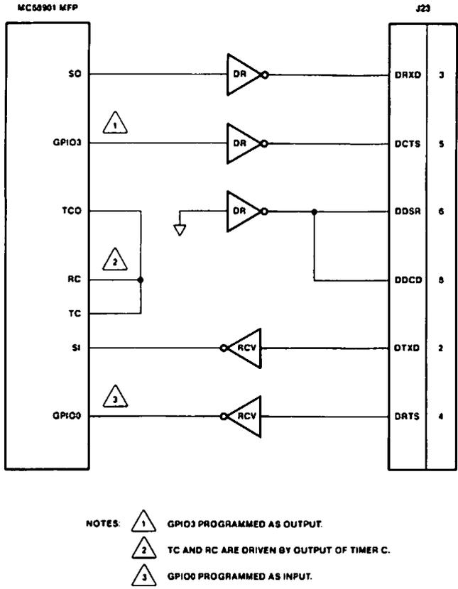
FIGURE 4-3. MVME133XT Debug Port (To Terminal Only)
