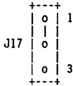
VMEbus IS TREATED AS D32 FOR THE PHYSICAL ADDRESS RANGE OF \$00400000 THROUGH \$FFFFFFF, AND AS D16 FOR PHYSICAL ADDRESS RANGE \$F0000000 THROUGH \$FFFFFFFF AND \$FFFF0000 THROUGH \$FFFFFFF. (FACTORY CONFIGURATION)
