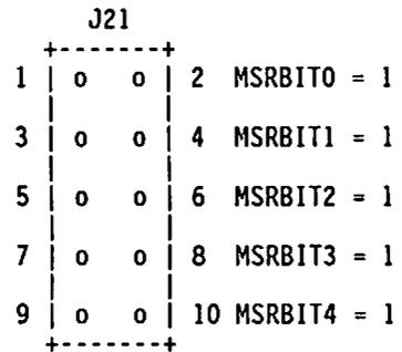
J21 is used to set five bits of the MSR. For details, refer to the MSR description in Chapter 4.
