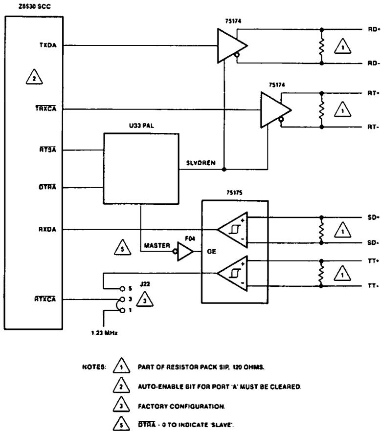
FIGURE 4-5. MVME133XT RS-485 Port Configured as Slave (To DTE)
