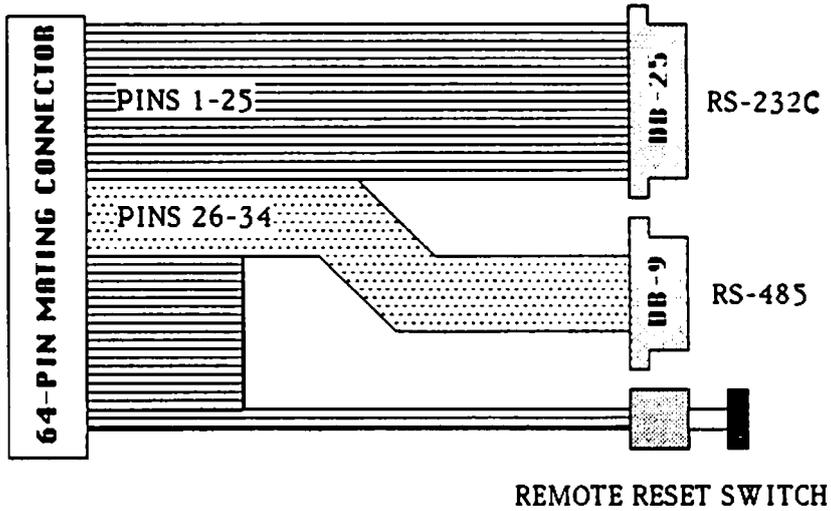
FIGURE 2-3. Cabling Connections to P2, Suggestion 2
