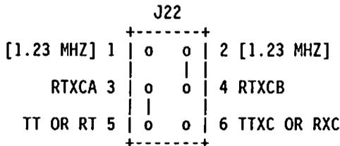
RTXCA IS DRIVEN BY TT+/- IF PORT A IS CONFIGURED AS A SLAVE, OR FROM RT+/- IF PORT A IS CONFIGURED AS A MASTER. RTXCB IS DRIVEN BY ONBOARD 1.230769 MHZ.
