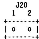
GLOBAL TIME-OUT DISABLED: THIS MAY CAUSE A SYSTEM PROBLEM. REFER TO PARAGRAPH 2.4.3. IN THIS CONFIGURATION, THE SYSTEM HANGS UP IF MVME133XT IS THE SYSTEM CONTROLLER AND THE SOFTWARE ATTEMPTS TO ACCESS A NON-EXISTENT VMEbus DEVICE.
