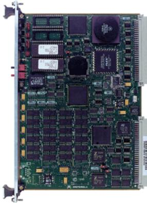
**VMEbus single-board computer that eliminates the need for additional backplane modules**
