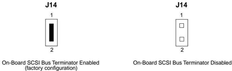
**Note** If the MVME162LX is to be used at one end of the SCSI bus, the SCSI bus terminators must be enabled.
