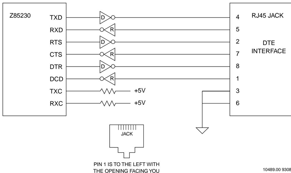
**Figure A-1. Serial Interface Connections**
