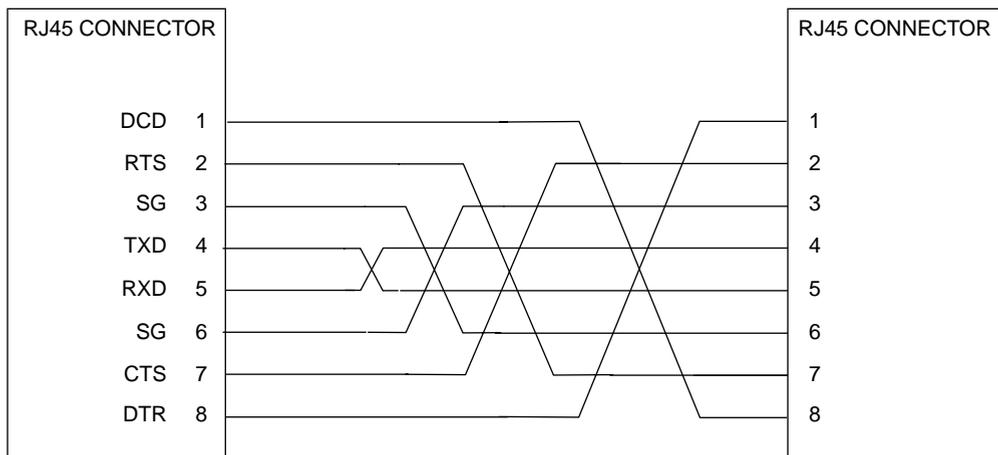
**Figure A-4. Typical RJ45 Serial Cable**
