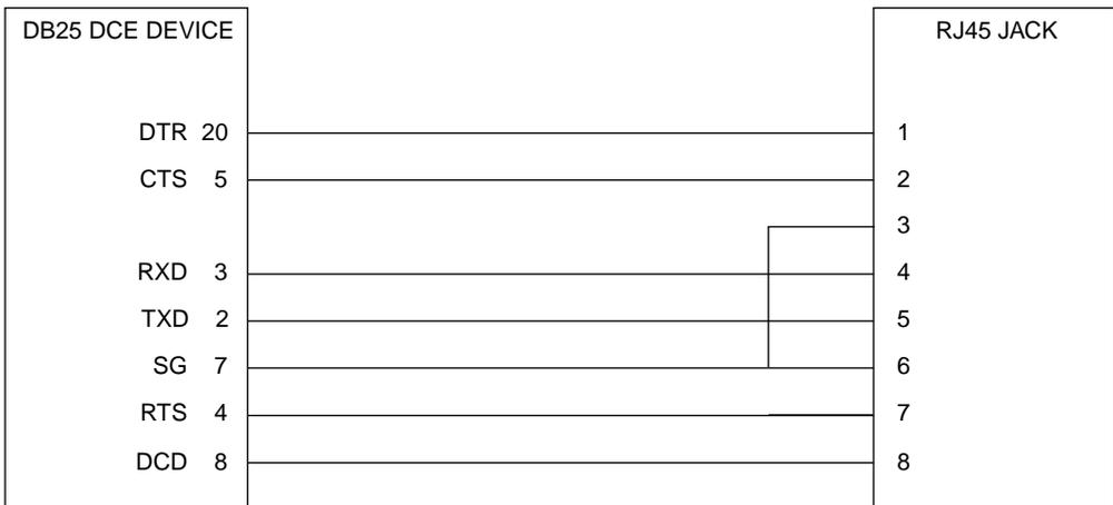
**Figure A-3. DB25-DCE-to-RJ45 Adapter**
