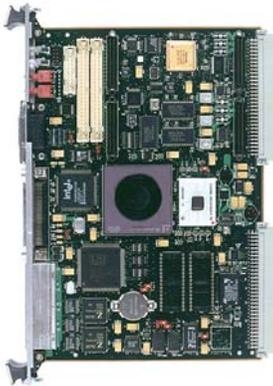
**Dual IndustryPack logic interface for embedded monitoring and control applications**
