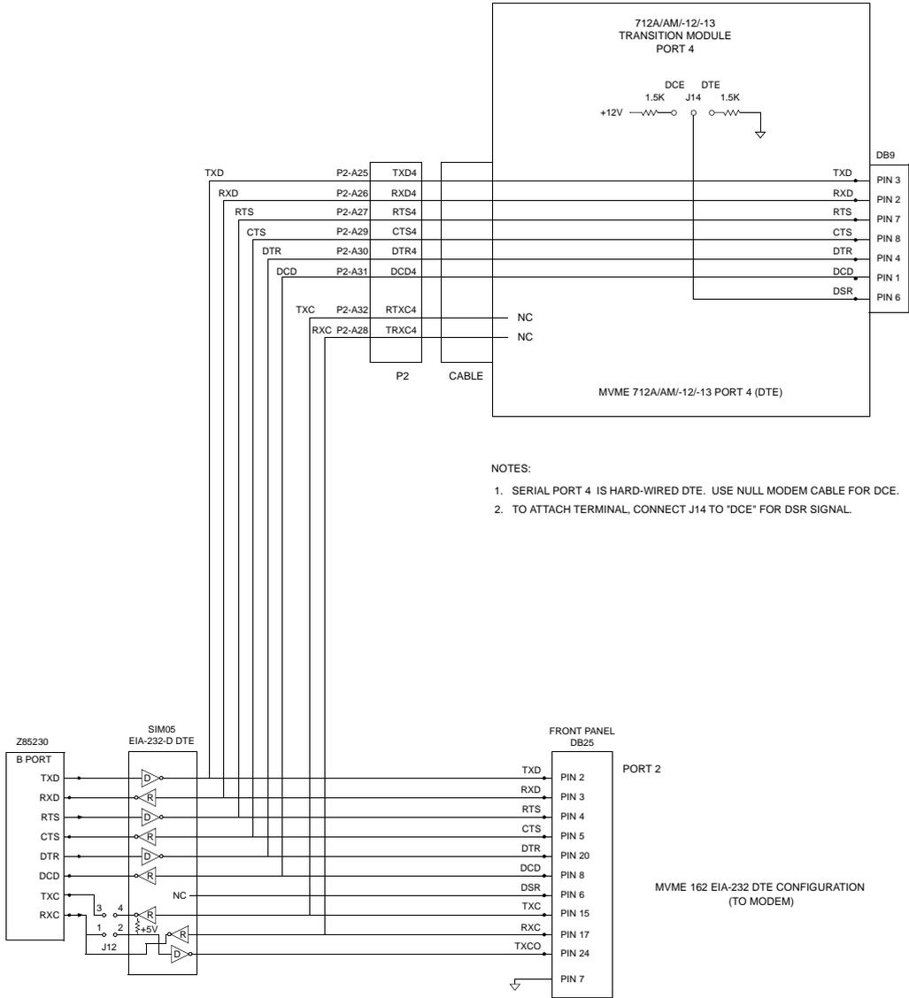
**Figure 2-5. MVME162FX EIA-232-D Connections, MVME712A/AM/-12/-13 (Sheet 3 of 4)**
