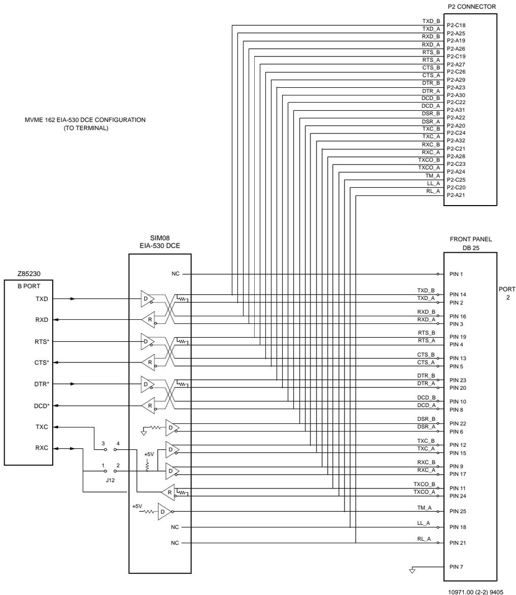
Figure 2-4. MVME162FX EIA-530 Connections (Sheet 2 of 2)
