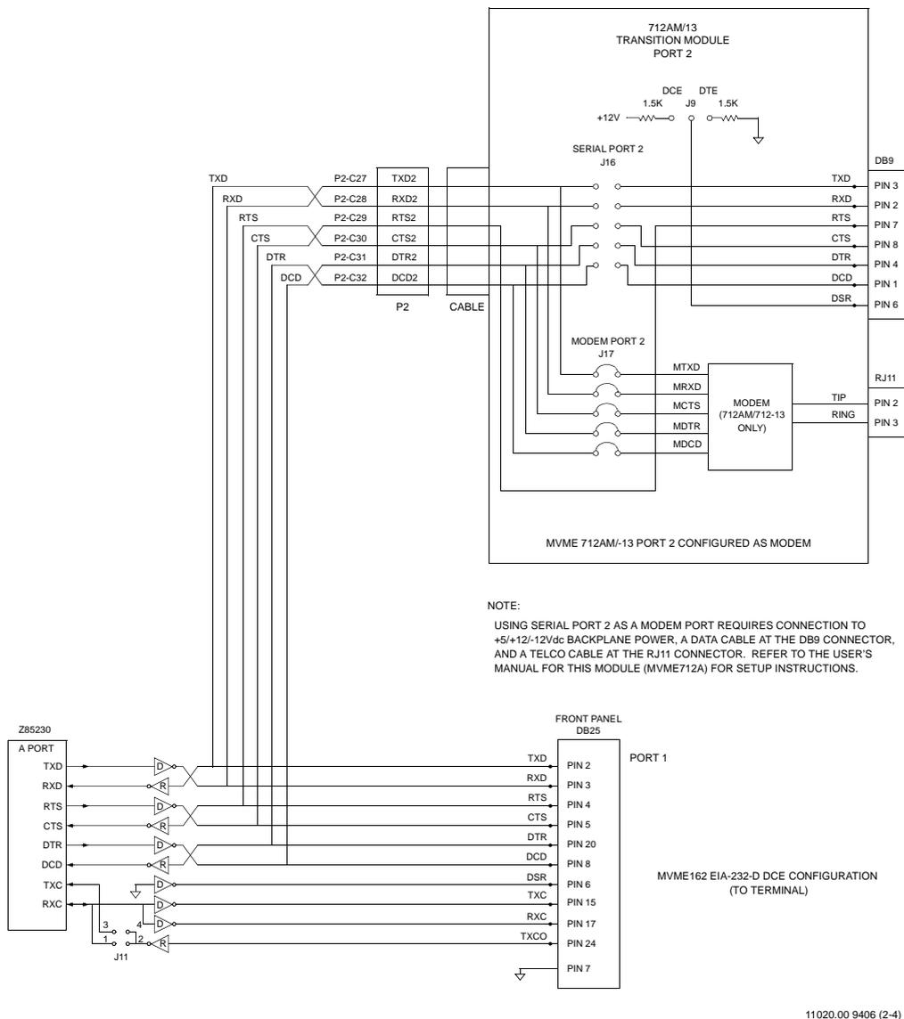
**Figure 2-5. MVME162FX EIA-232-D Connections, MVME712A/AM-12/13 (Sheet 2 of 4)**
