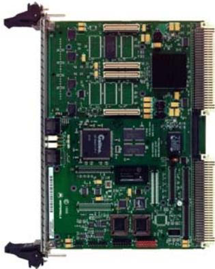
**Modular single-board computer providing high-performance expansion I/O**
