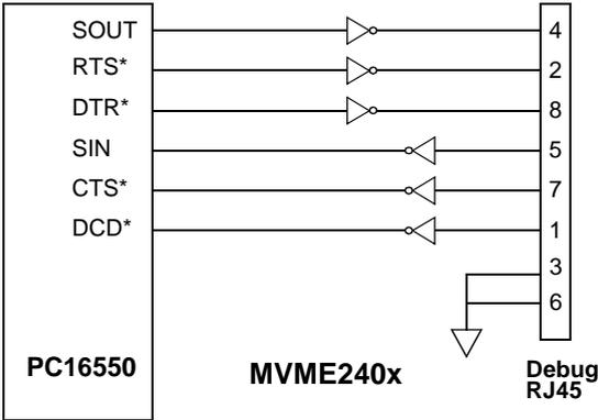
Figure 2-1. MVME240x DEBUG Port Configuration
