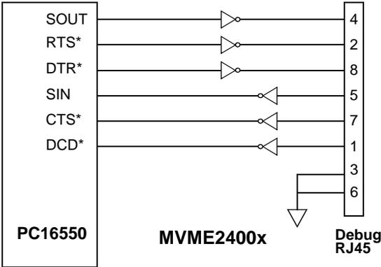
Figure 2-2. MVME2400x DEBUG Port Configuration
