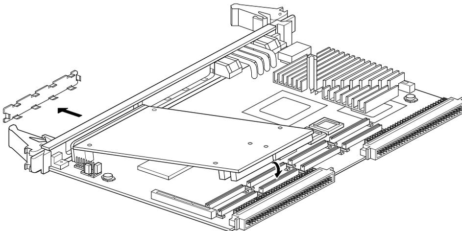
**Figure 1-3. Typical Single-width PMC Module Placement on MVME2400x**
