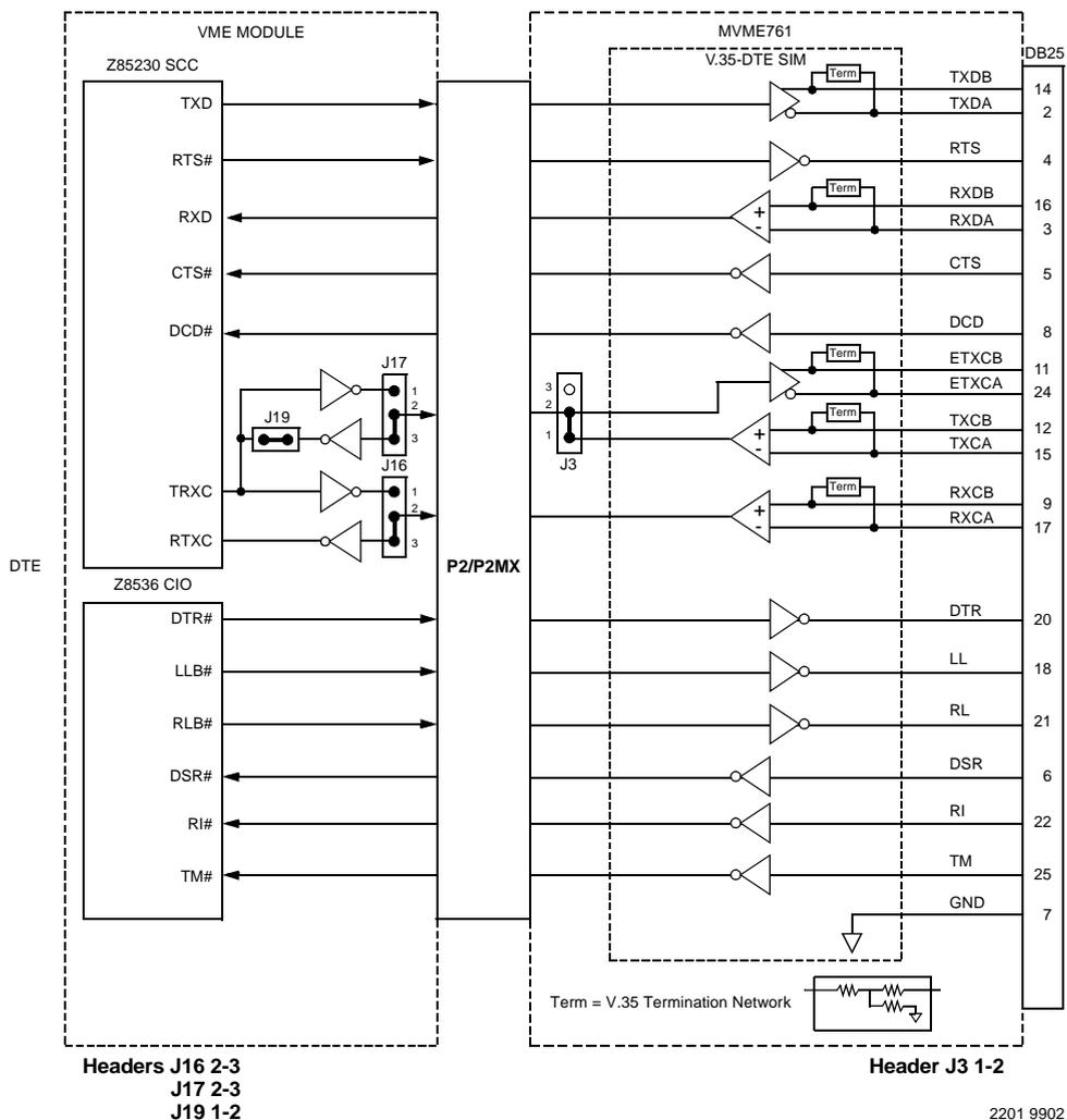
Figure 1-25. MVME761 V.35-DTE Configuration Port 4
