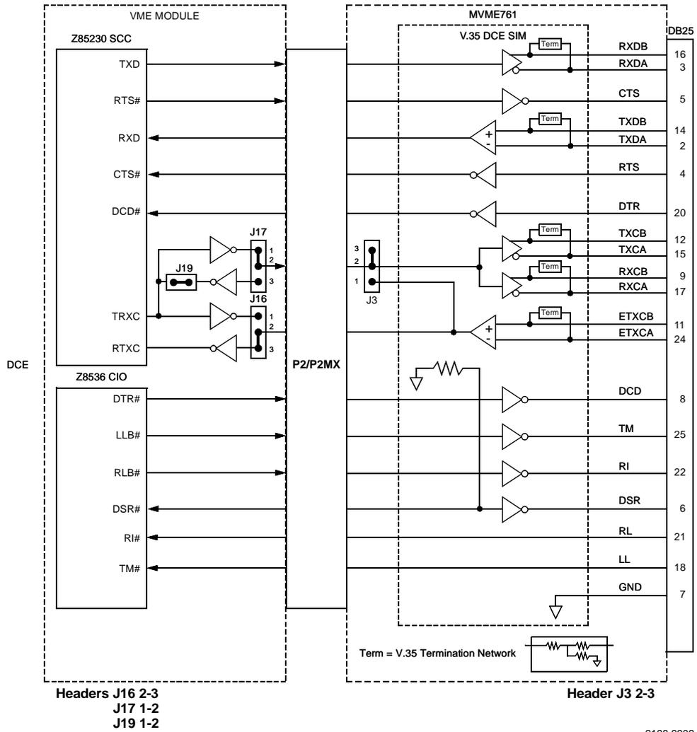
Figure 1-24. MVME761 V.35-DCE Configuration Port 4
