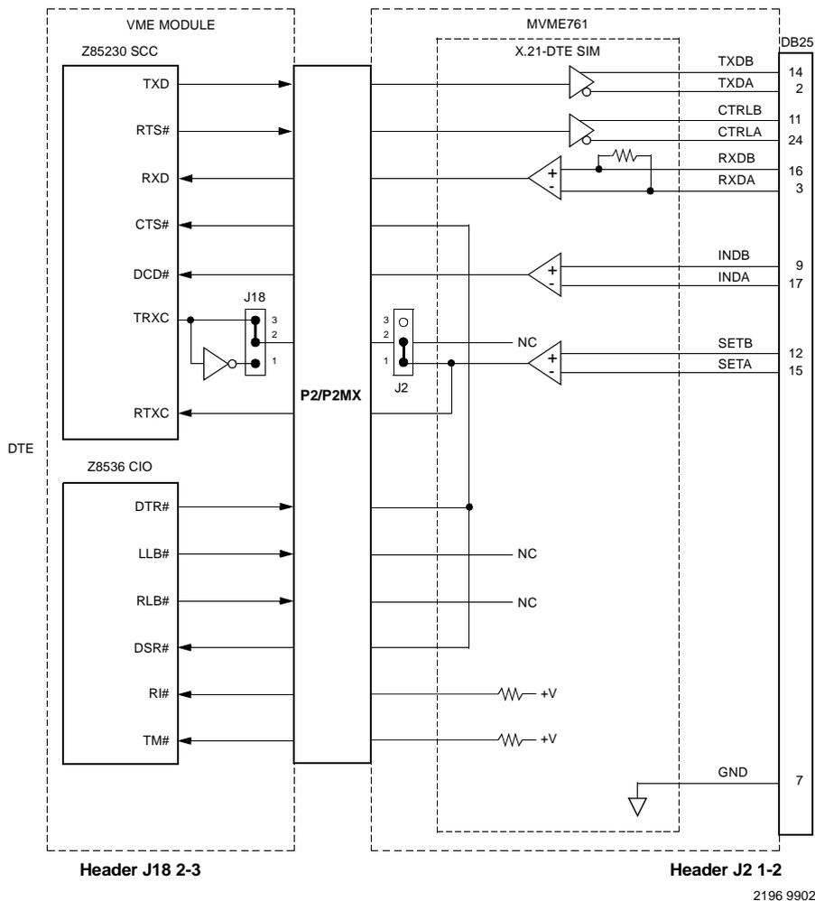
Figure 1-27. MVME761 X.21-DTE Configuration Port 3
