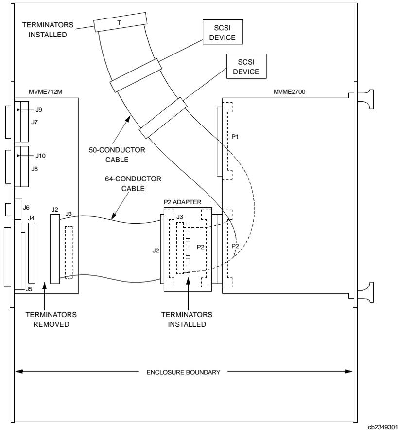
**Figure 1-23. MVME712M/MVME2700 Cable Connections**
