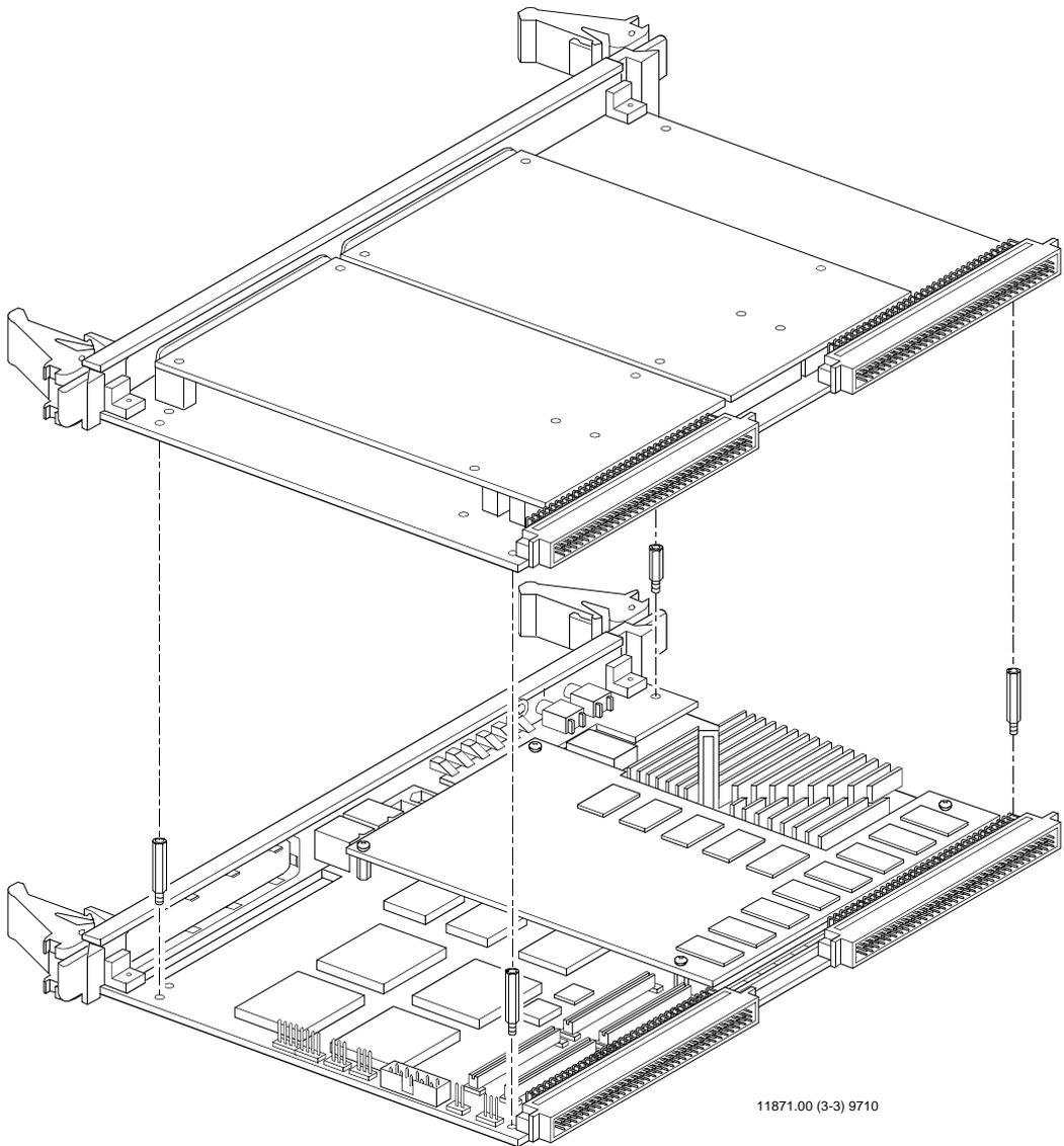
**Figure 1-22. PMC Carrier Board Placement on MVME2700**
