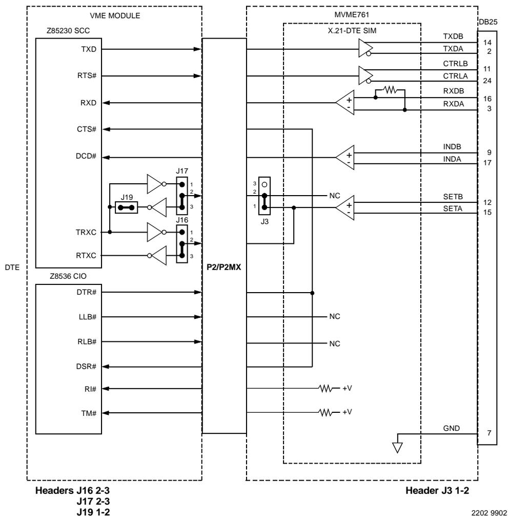
Figure 1-29. MVME761 X.21-DTE Configuration Port 4
