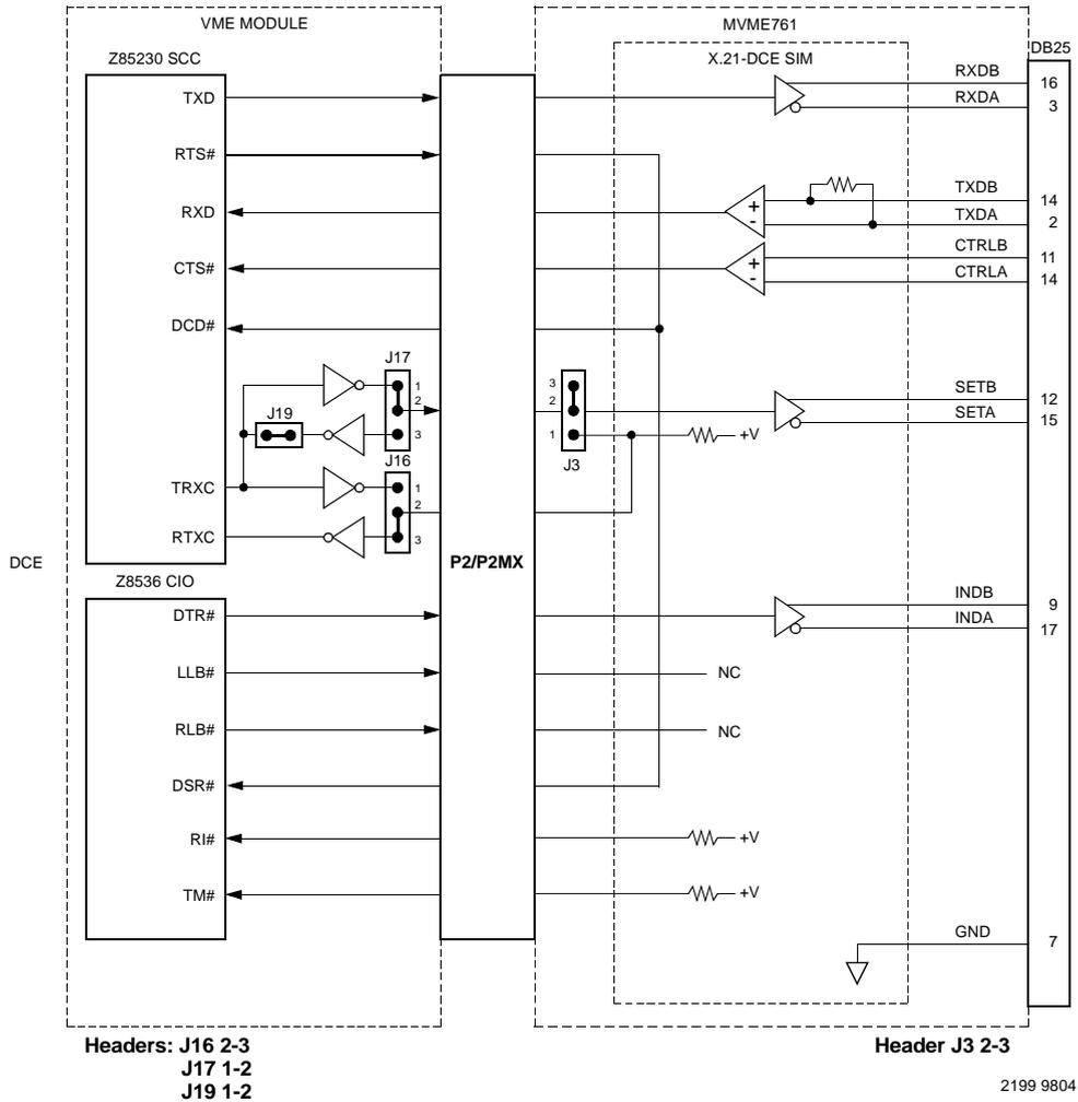
Figure 1-28. MVME761 X.21-DCE Configuration Port 4
