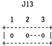
USES ONBOARD 16 MHz
