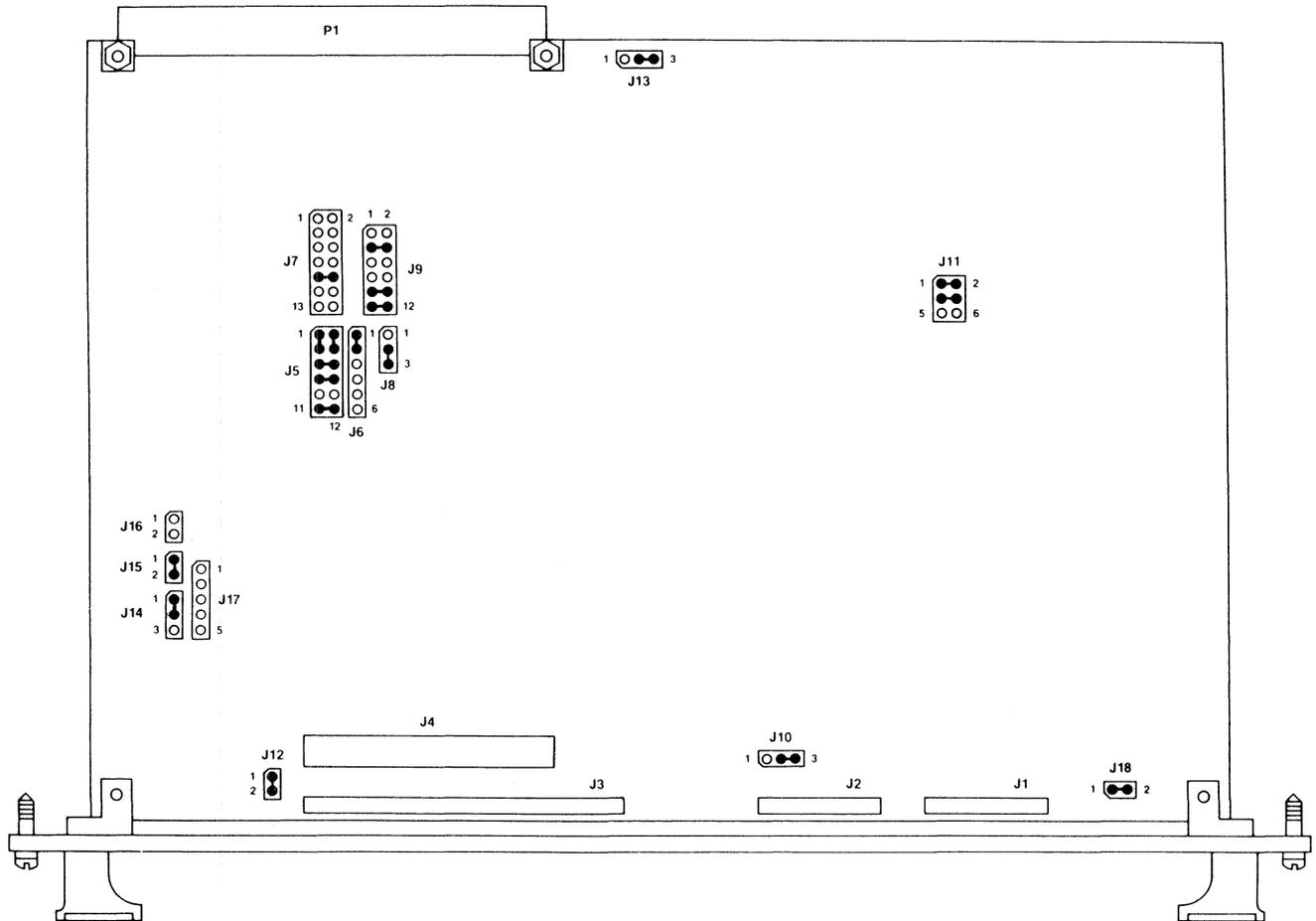
FIGURE 2-1. MVME320B Connector and Header Locations
