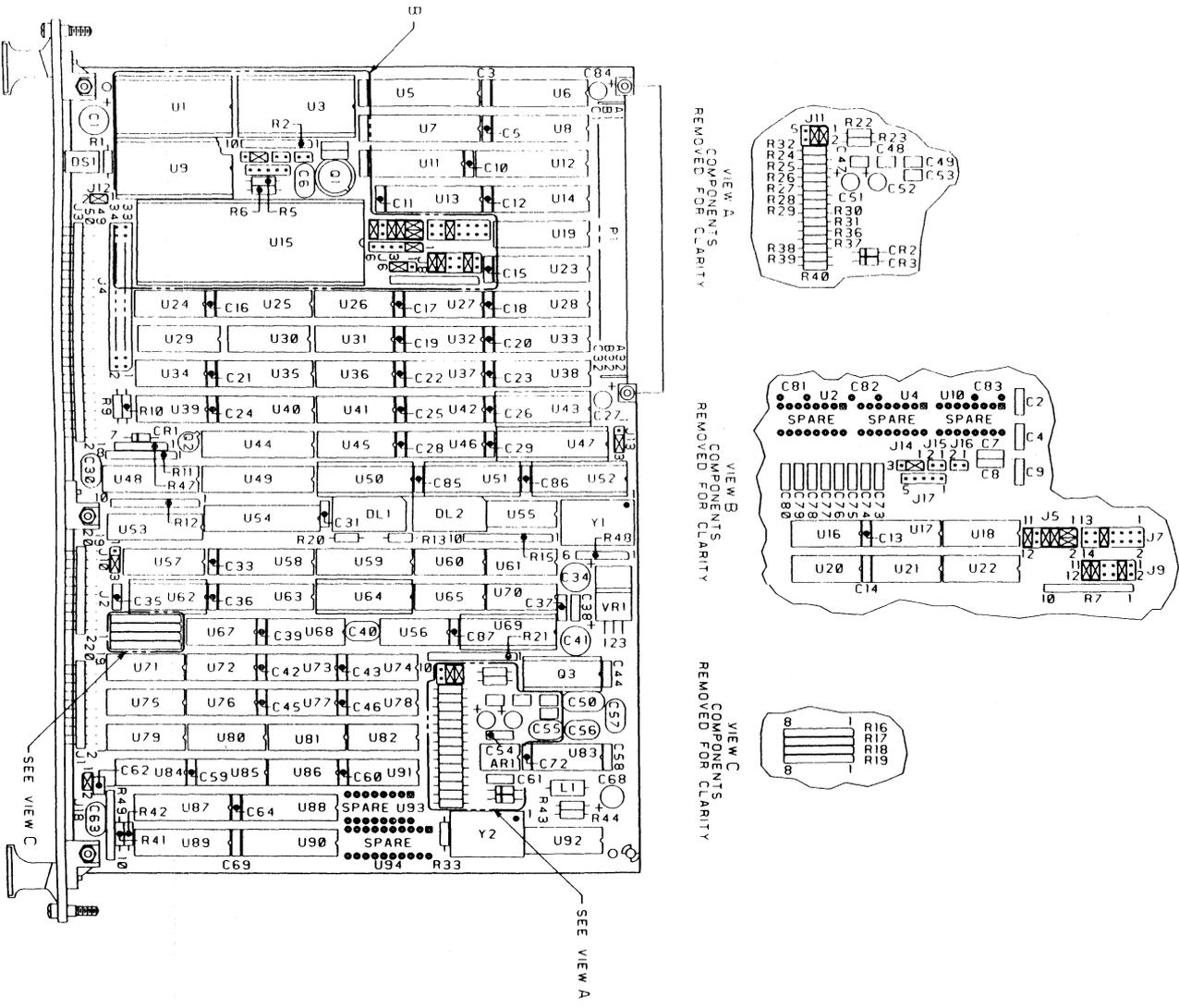
FIGURE 13-1. MWME320B Parts Location Diagram (Sheet 1 of 2)
