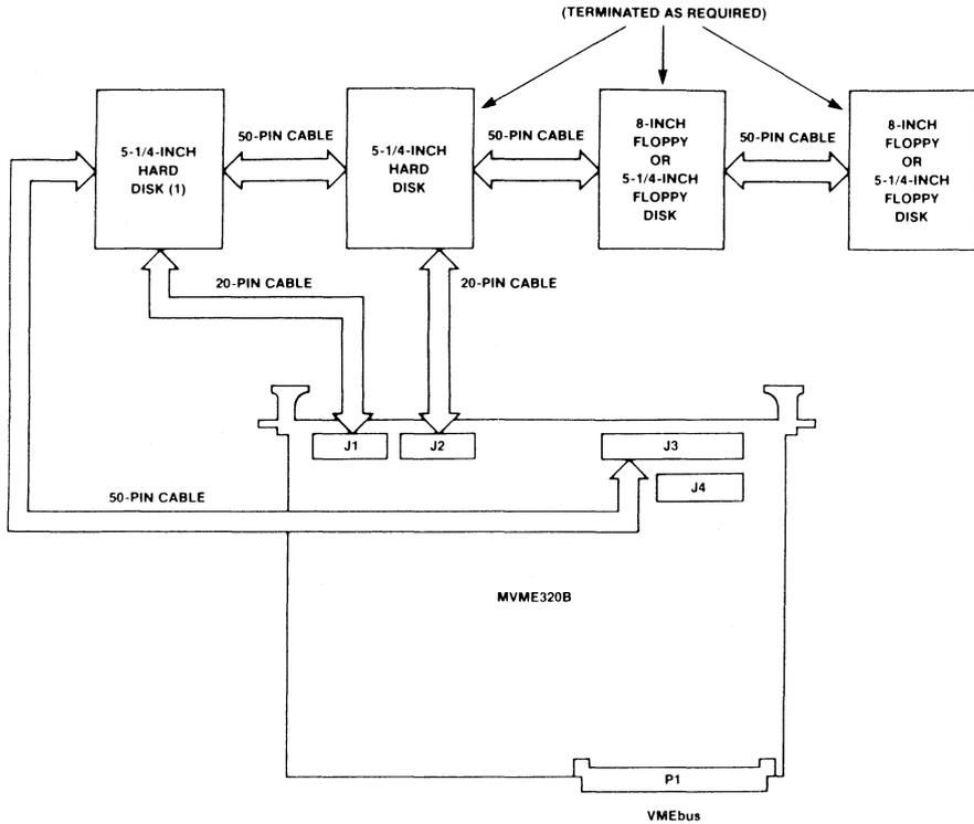
NOTES: (1) Only the end of each signal line requires termination. For systems mixing 5-1/4 inch and 8-inch drives, this can be accomplished by using an 8-inch drive as the last drive installed and terminating all signal lines on that drive.
