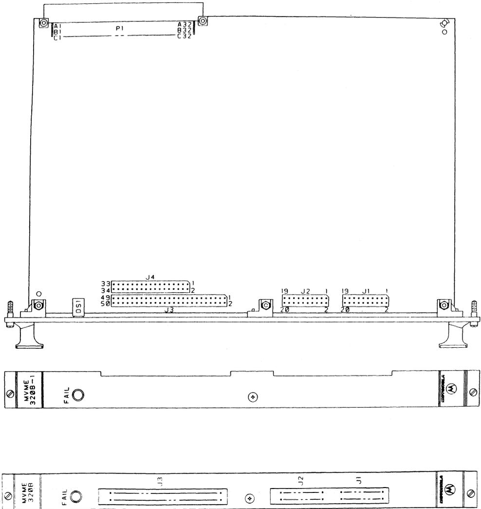
FIGURE 13-1. MVME320B Parts Location Diagram (Sheet 2 of 2)
