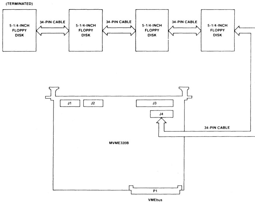
NOTE: 1. Only the end of each signal line (typically on the last drive) requires termination.
