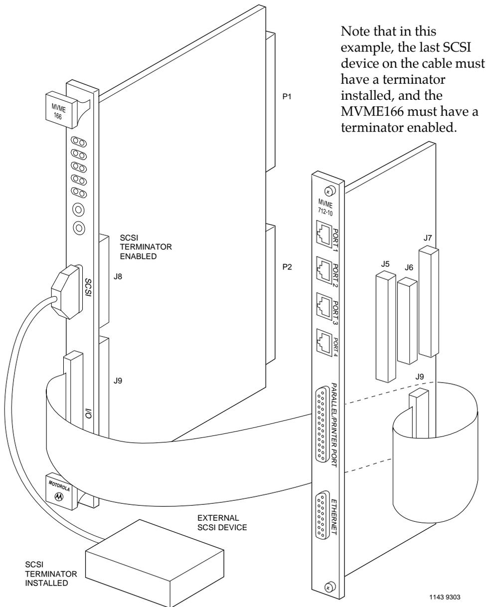
**Figure 2-5. Typical MVME712-10 Installation at Front of Chassis**
