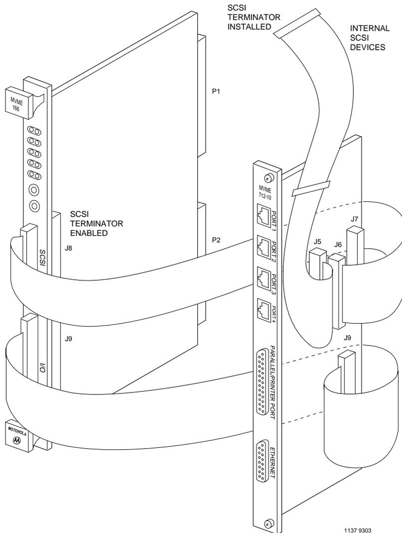
Note that in this example, the last SCSI device on the cable must have a terminator installed, and the MVME166 must have a terminator enabled. No terminator would be required on the MVME712-10.
