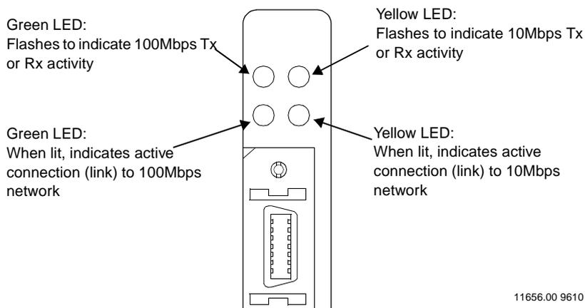
**Figure 4-2. LEDs on the XRPMC100BT Front Panel**
