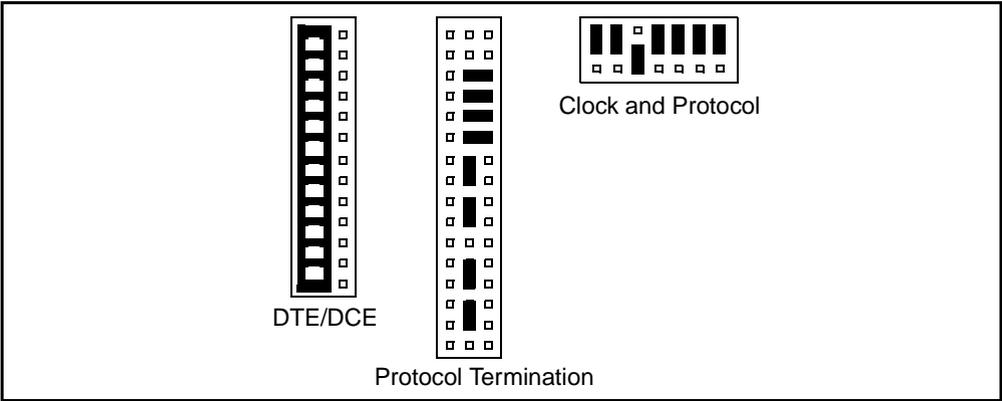
Transition Module Jumpers (DCE Type, EIA232 Protocol, DCE Clocking, DTE Transmit Data)
