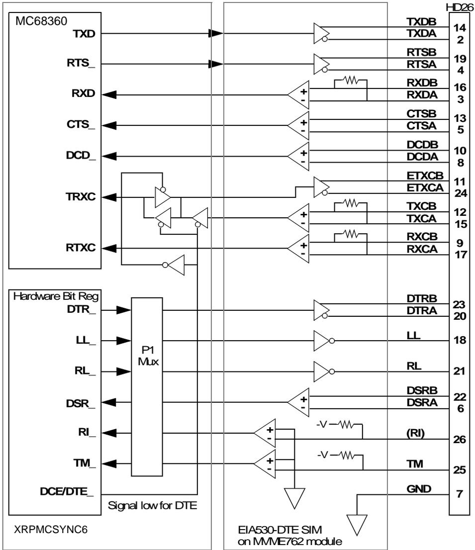
Figure 6-10. EIA530-DTE Serial Port Configuration
