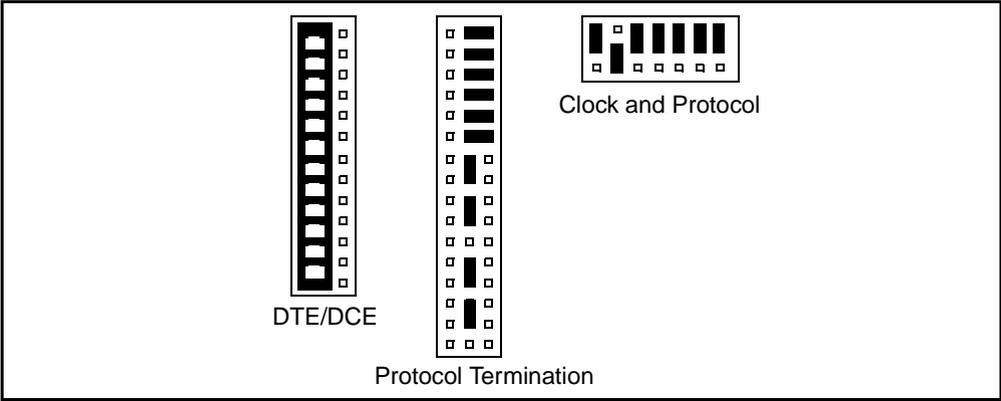
Transition Module Jumpers (DCE Type, EIA422 Protocol, DCE Clocking, DTE Transmit Data)
