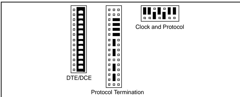
Transition Module Jumpers (DTE Type, EIA232 Protocol, DTE Clocking
