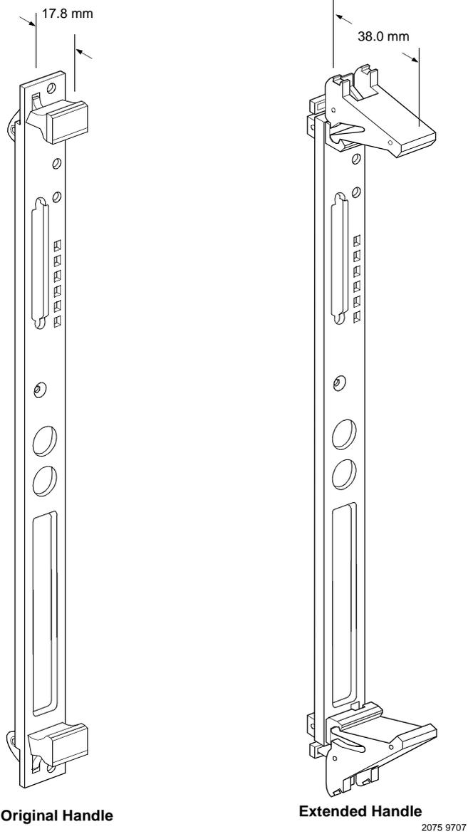
**Figure A-1. Original and Extended Injector Handles**
