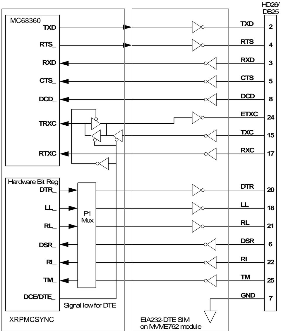
Figure 6-8. EIA232-DTE Serial Port Configuration
