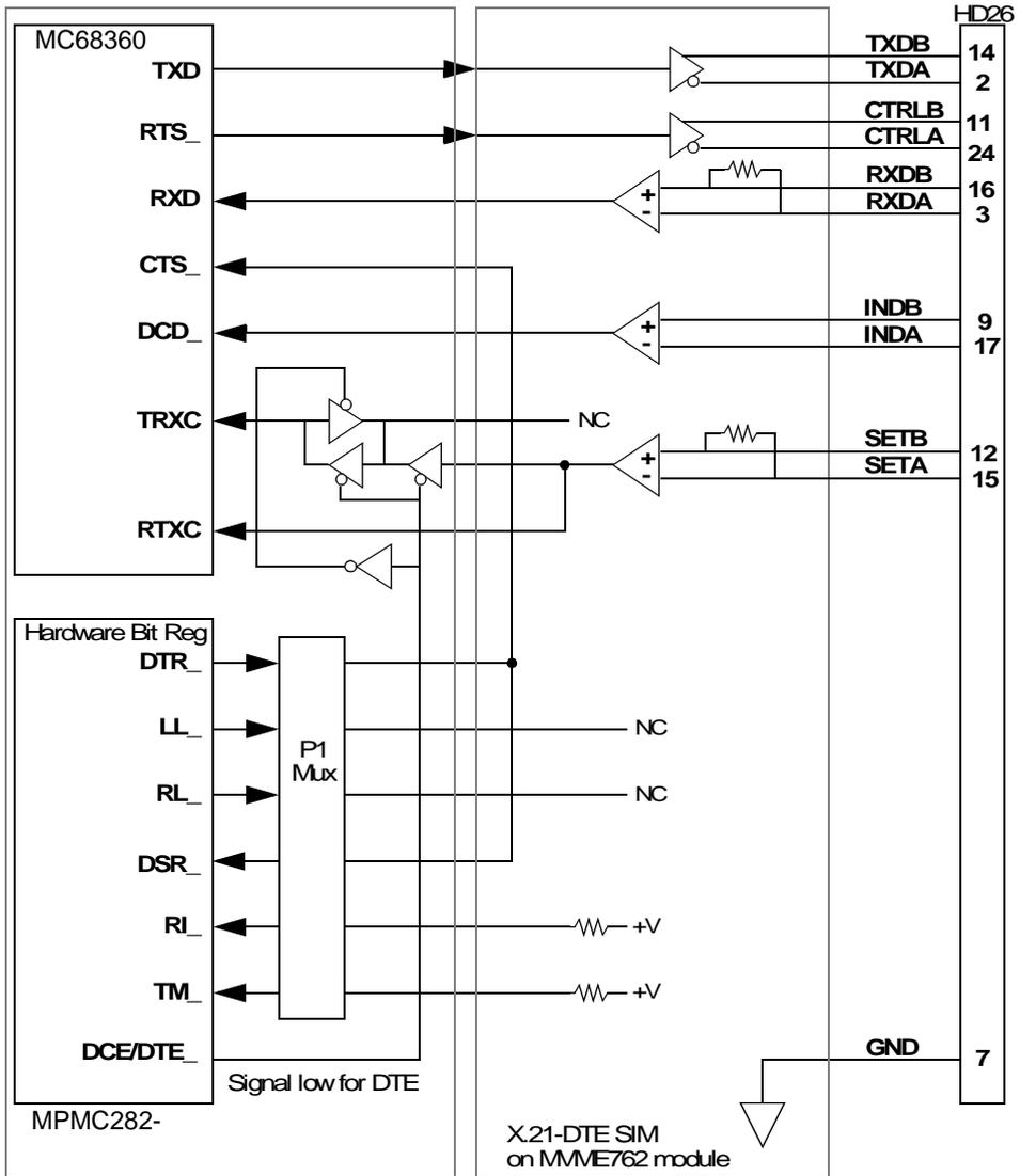
Figure 5-11. X.21-DTE Serial Port Configuration
