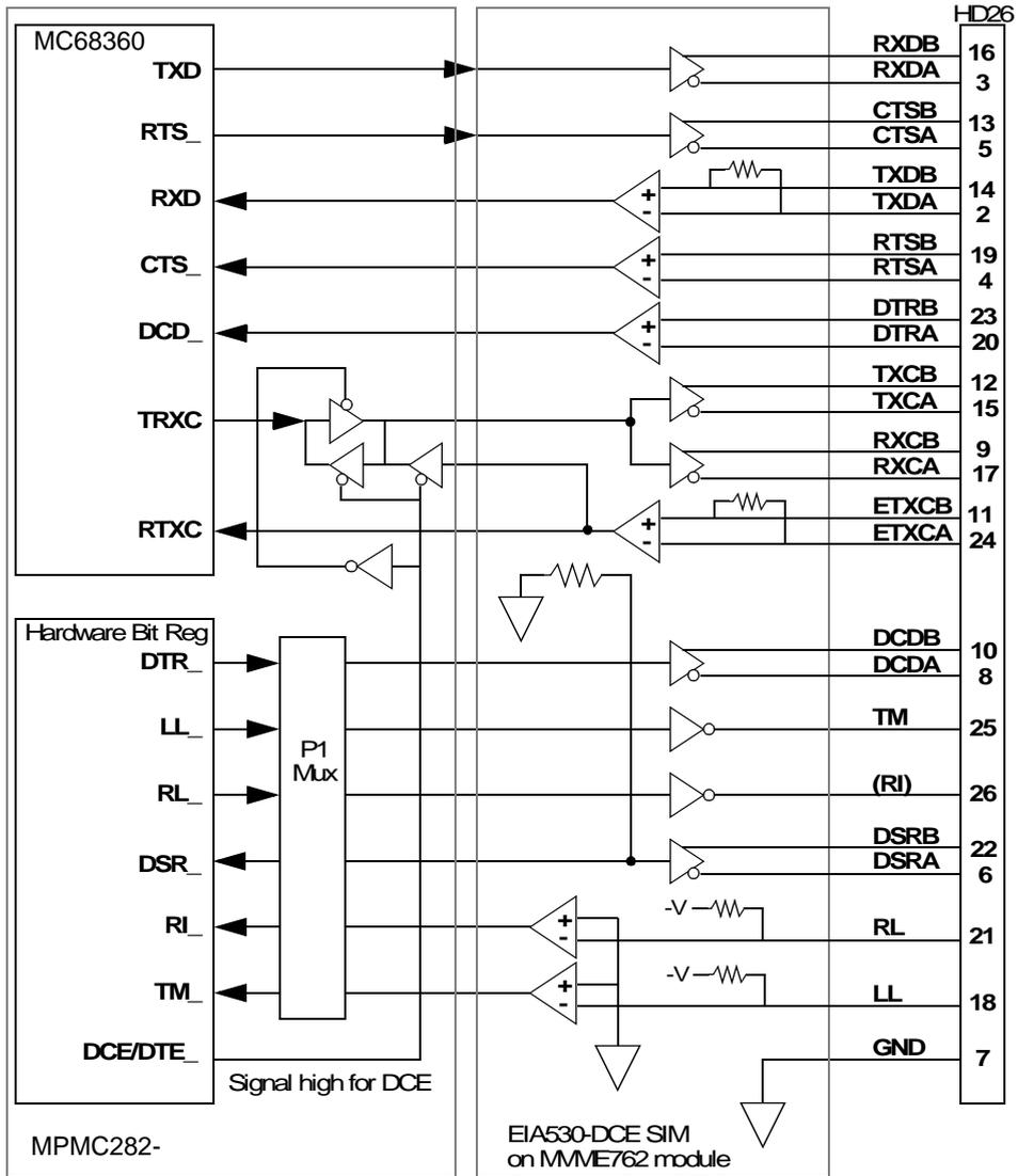
Figure 5-6. EIA530-DCE Serial Port Configuration
