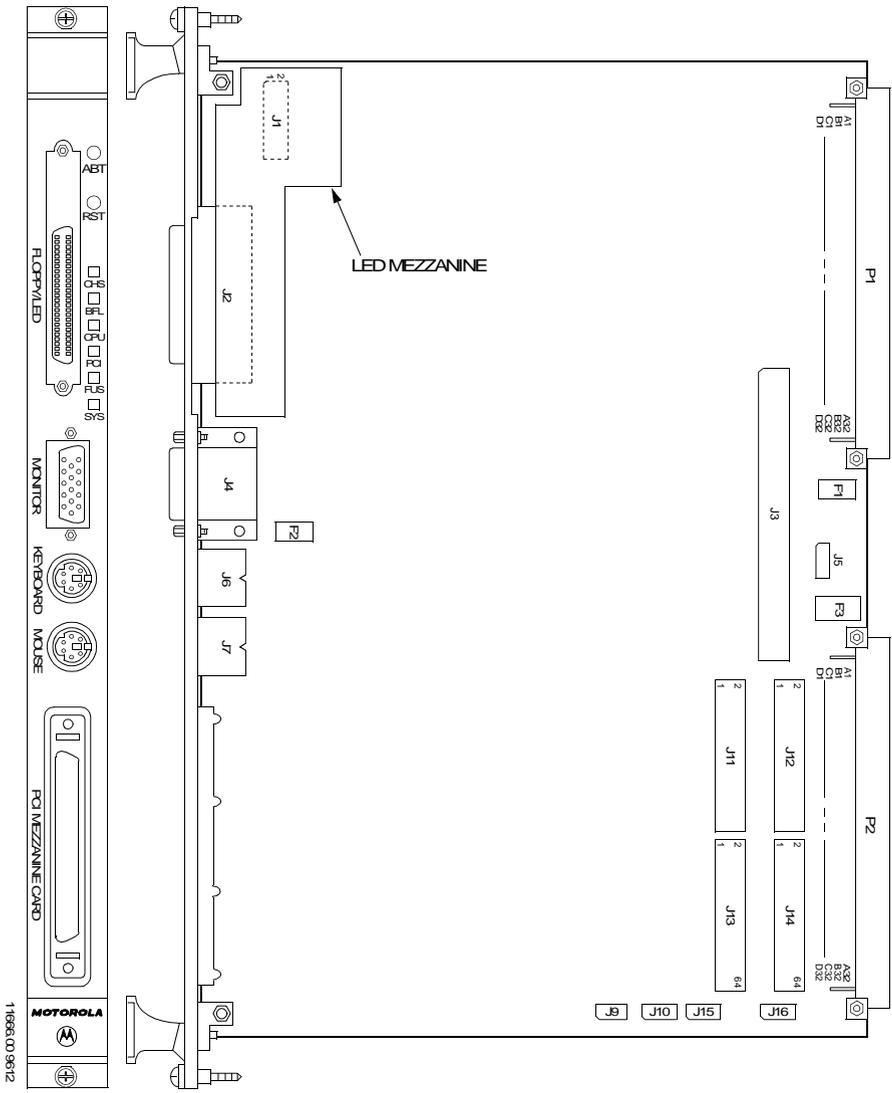
Figure 3-4. Base Board Switches, Headers, Connectors, Fuses, LEDs
