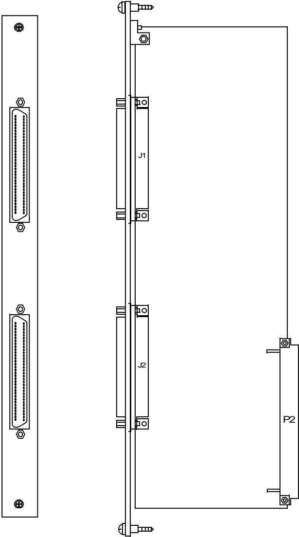
Figure 6-5. MVME712-104 SCSI Drive Transition Module
