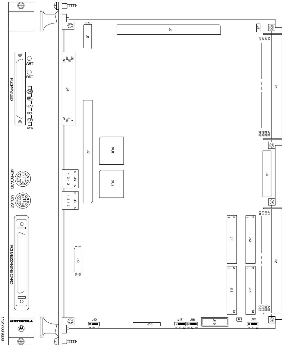
Figure 3-2. XR603E-1X/604E-1X Switches, Headers, Connectors, Fuses, LEDs
