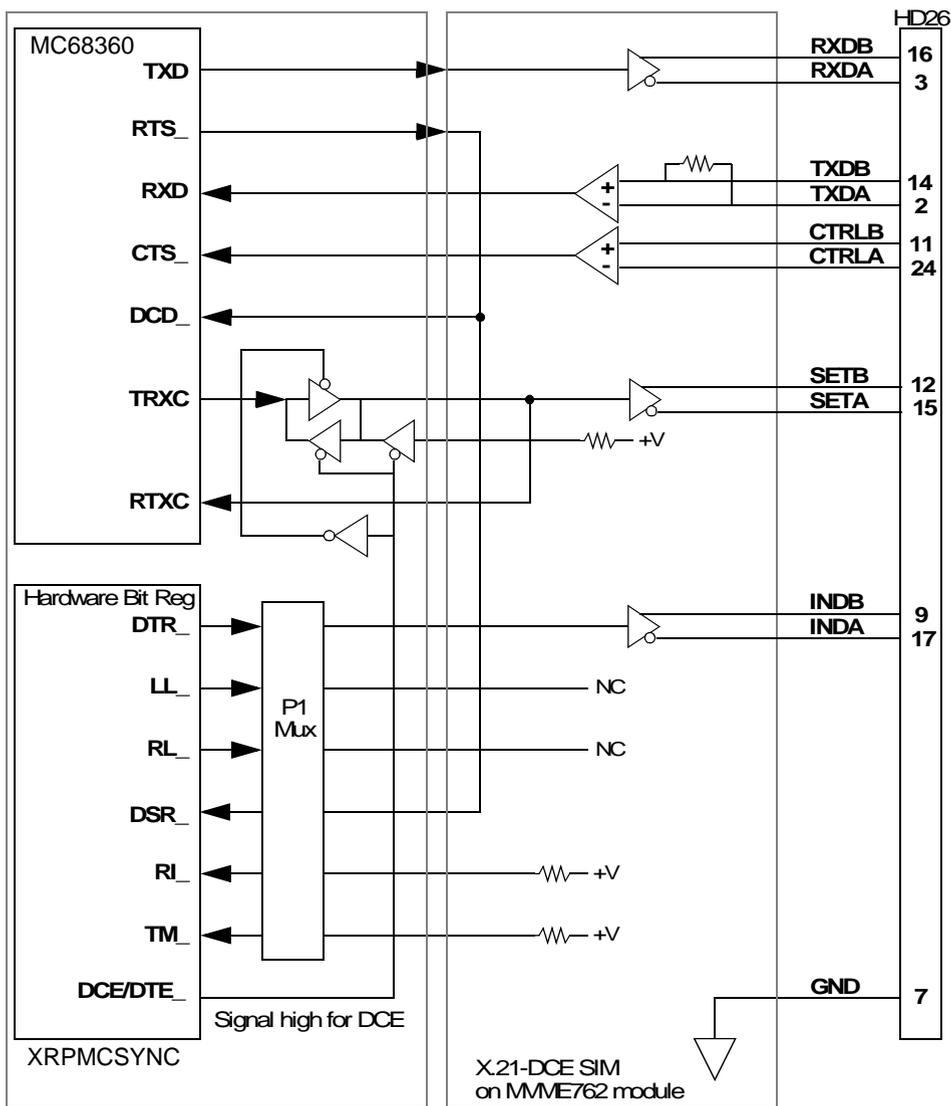
Figure 6-13. X.21-DCE Serial Port Configuration
