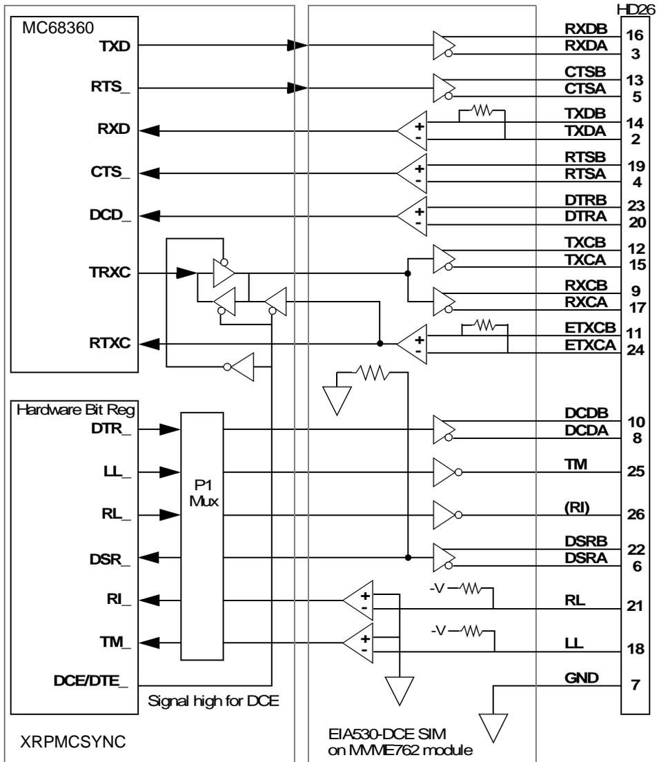
Figure 6-9. EIA530-DCE Serial Port Configuration
