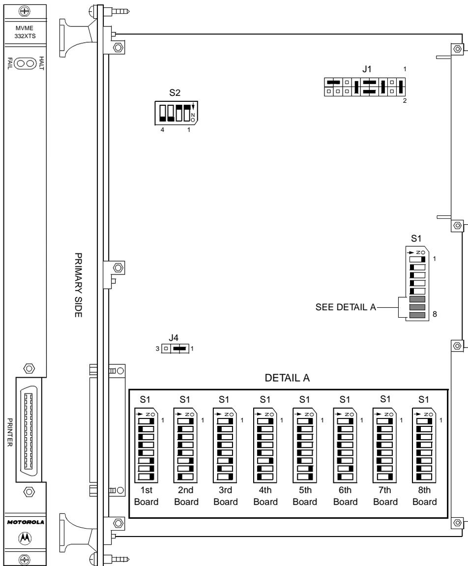
Figure 5-1. MVME332XTS Jumper and Switch Settings
