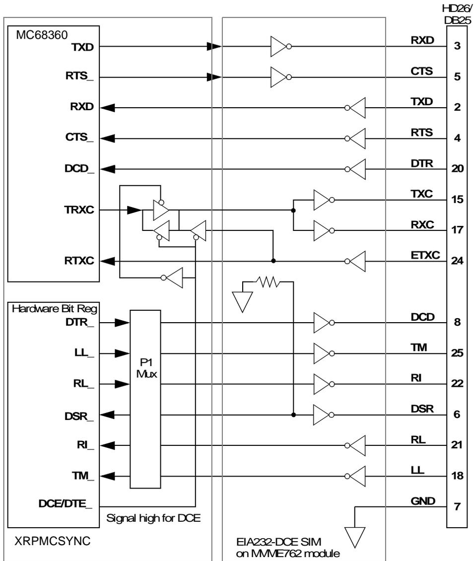
Figure 6-7. EIA232-DCE Serial Port Configuration
