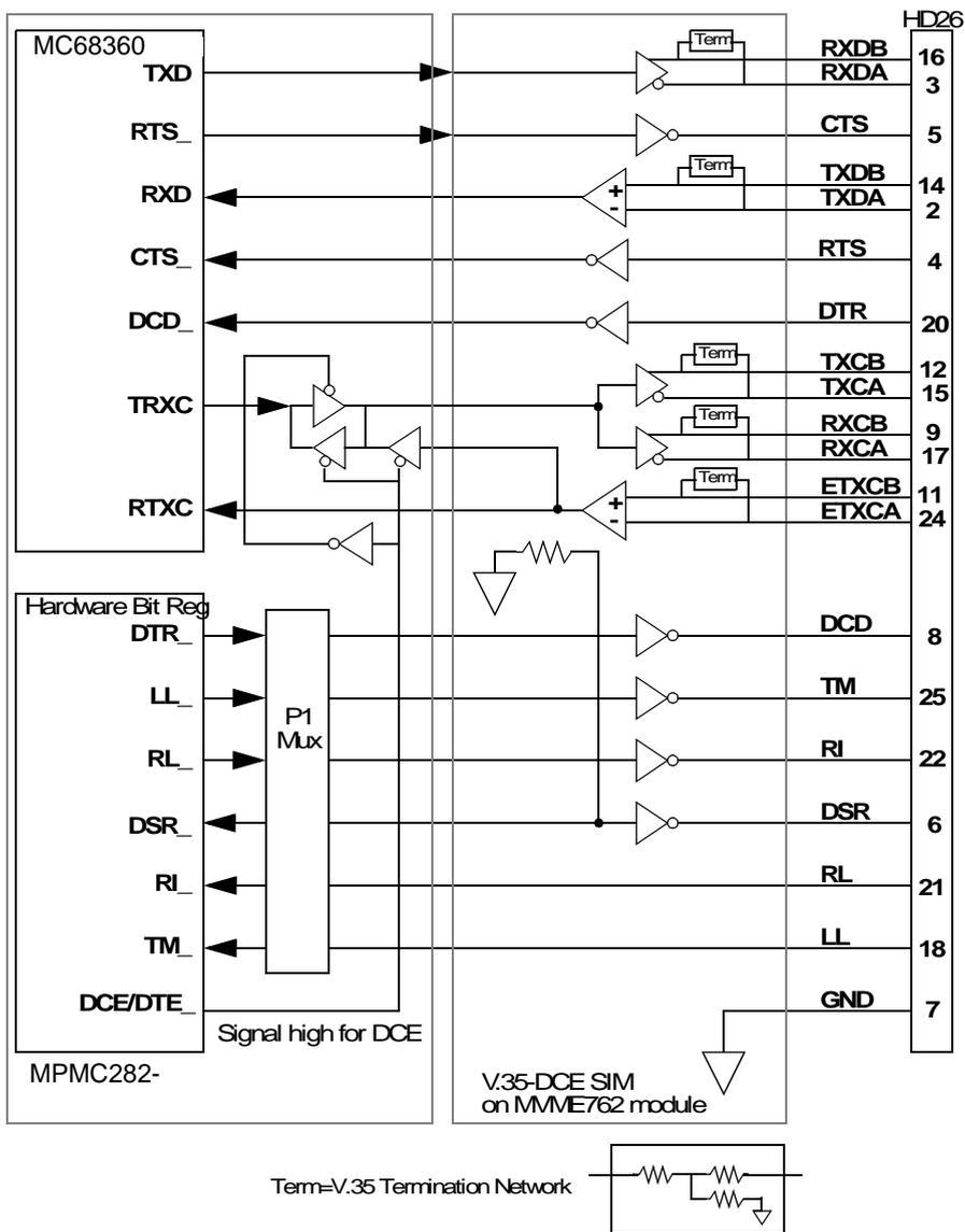
Figure 5-8. V.35-DCE Serial Port Configuration
