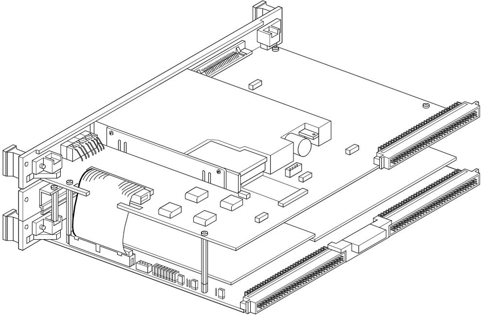
**Figure 2-2. Floppy Module Cabled and Attached to Dual-Slot CPU Board**
