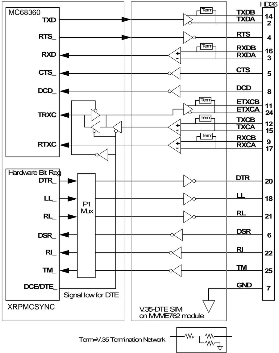
Figure 6-12. V.35-DTE Serial Port Configuration
