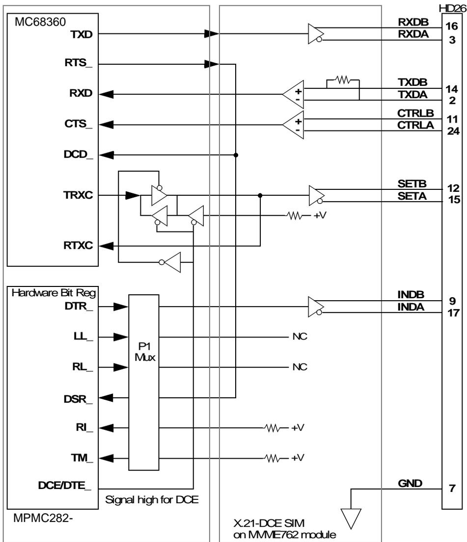
Figure 5-10. X.21-DCE Serial Port Configuration
