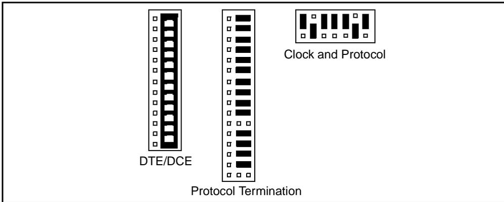
Transition Module Jumpers (DTE Type, EIA422 Protocol, DCE Clocking DTE Transmit Data)
