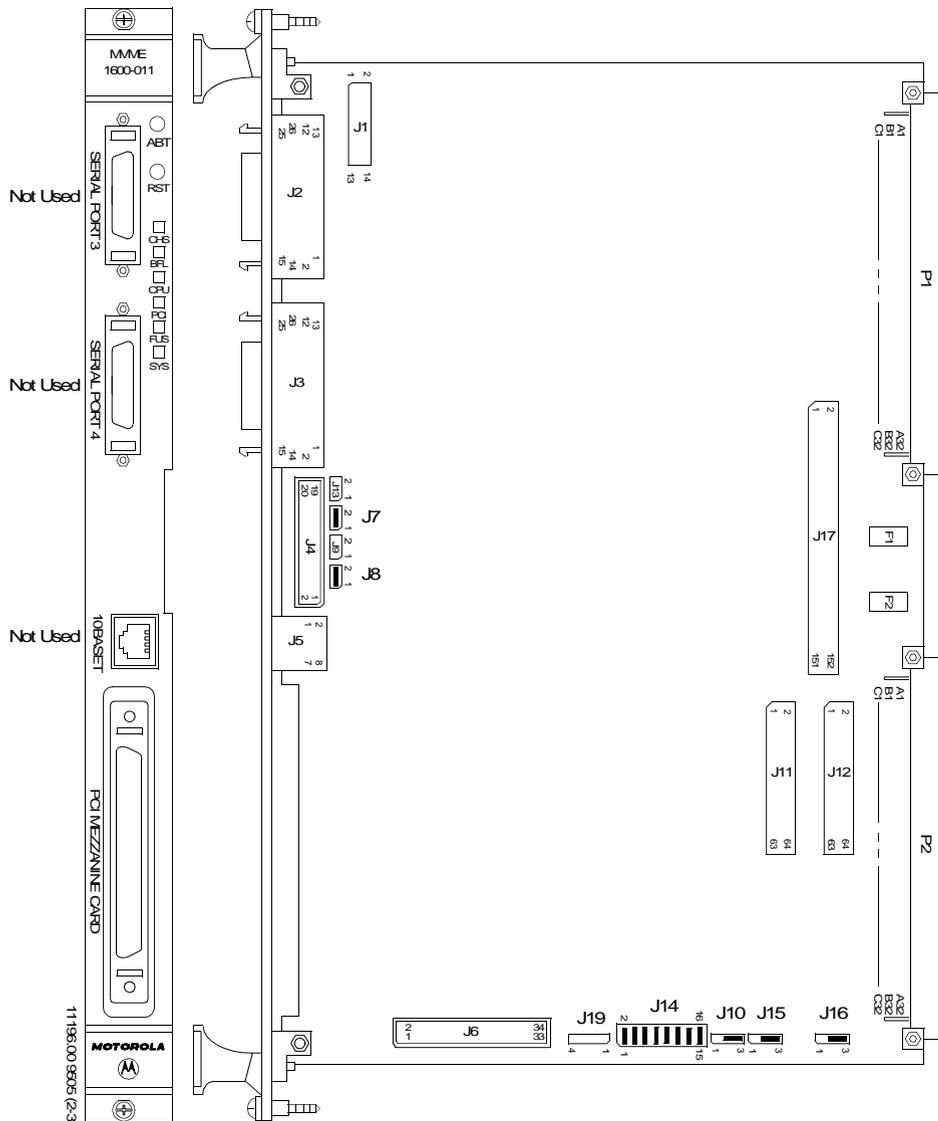
Figure 3-1. XR603-1P/603E-1P/604-1P Switches, Headers, Connectors, Fuses, LEDs
