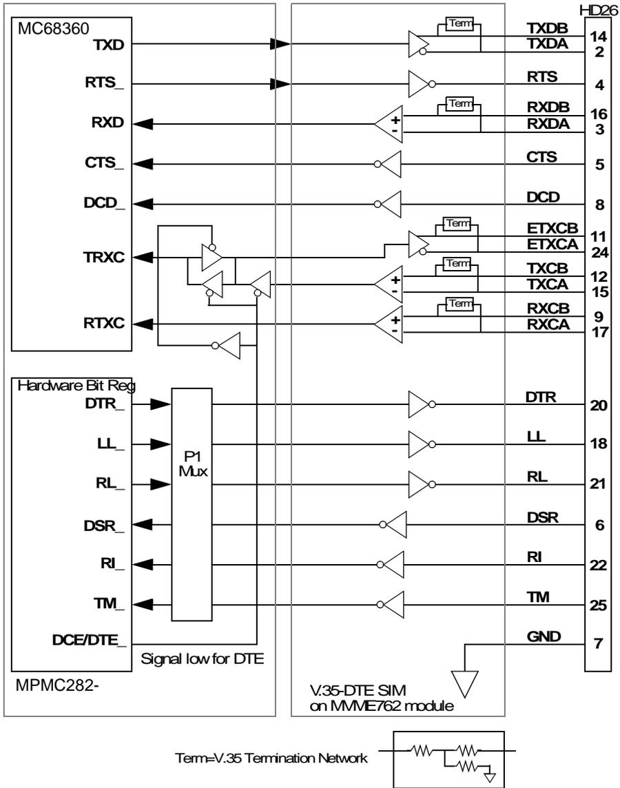
Figure 5-9. V.35-DTE Serial Port Configuration
