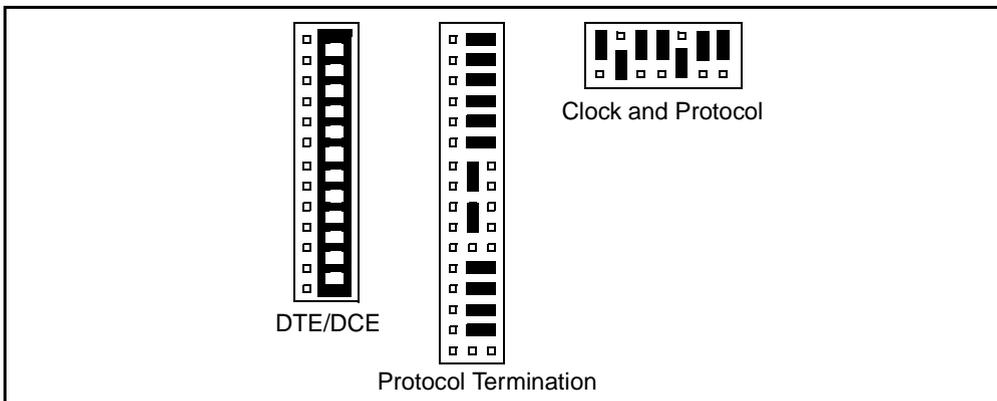
Transition Module Jumpers (DTE Type, EIA422 Protocol, DTE Clocking DTE Transmit Data)
