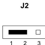
Flash Bank A Enabled (4MB/8MB, Soldered)
