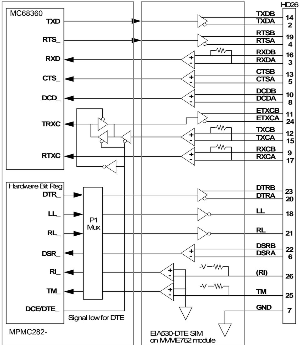
Figure 5-7. EIA530-DTE Serial Port Configuration
