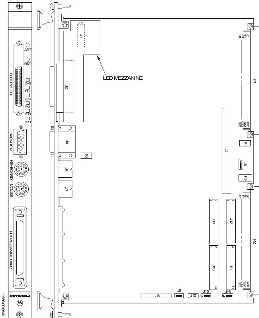
Figure 3-3. XR604E-1D Switches, Headers, Connectors, Fuses, LEDs
