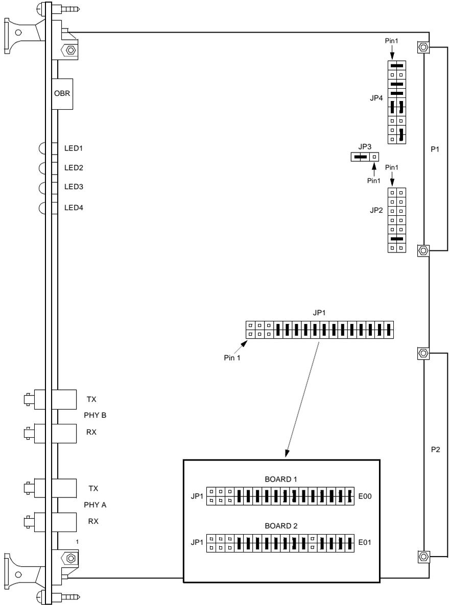
Figure 5-12. XR386-ST Board Layout
