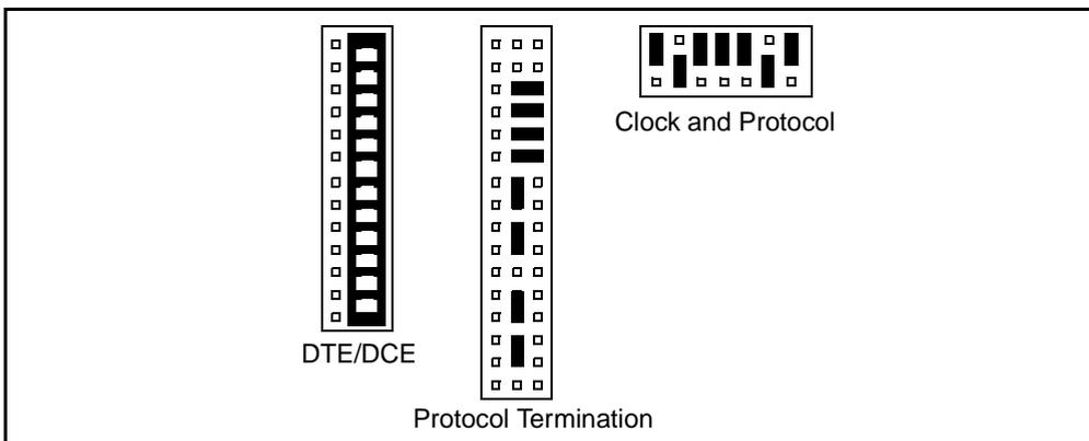
Transition Module Jumpers (DTE Type, EIA232 Protocol, DCE Clocking
