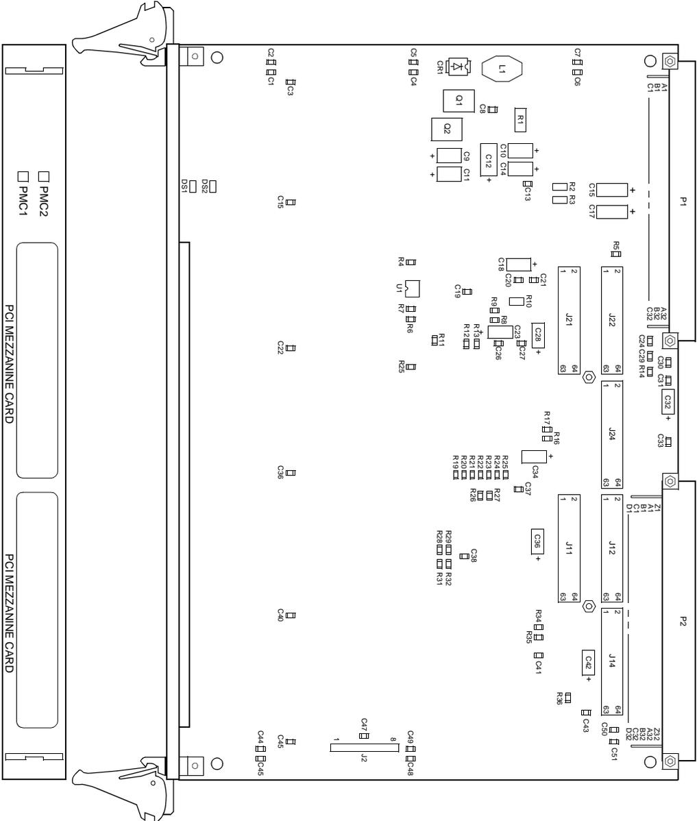
Figure 5-16. XRPMCEXP2 PMC Expansion Carrier
