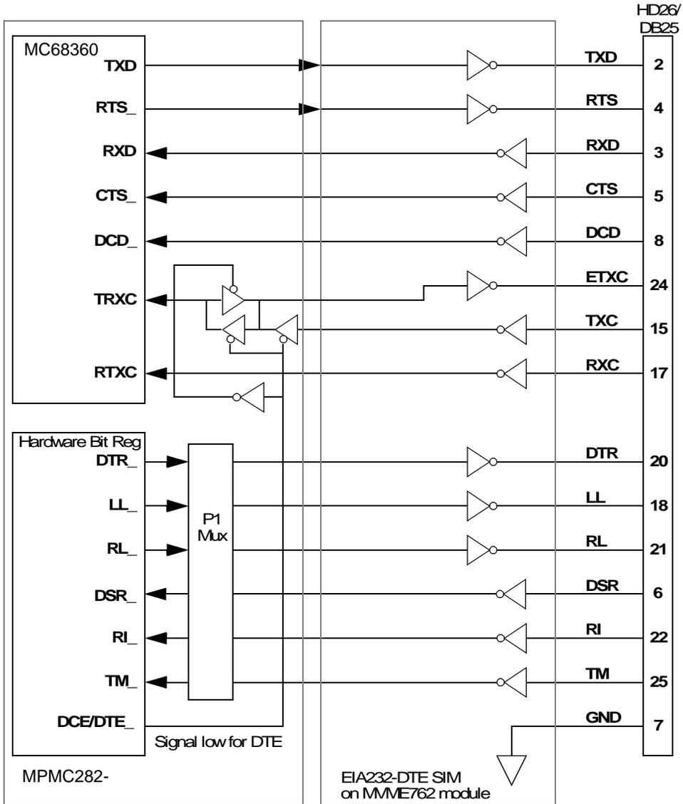
Figure 5-5. EIA232-DTE Serial Port Configuration
