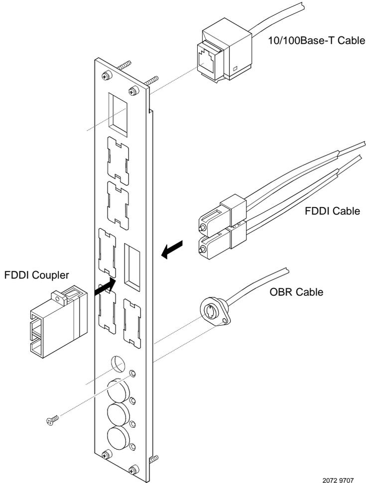
**Figure 6-25. The XRPMCLANPANL Transition Panel**
