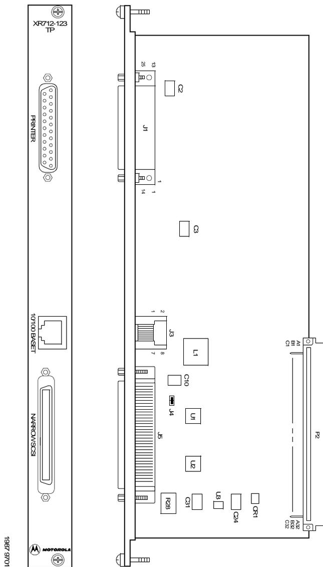
Figure 6-18. XR712-123TP Transition Module
