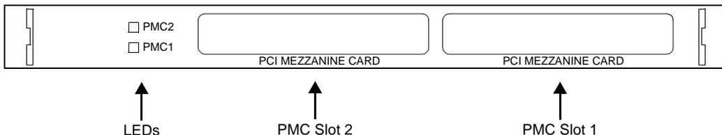
**Figure 5-14. Front Panel of the XRPMCEXP1 and XRPMCEXP2**
