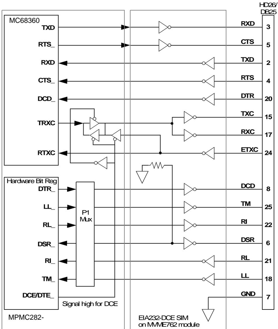
Figure 5-4. EIA232-DCE Serial Port Configuration
