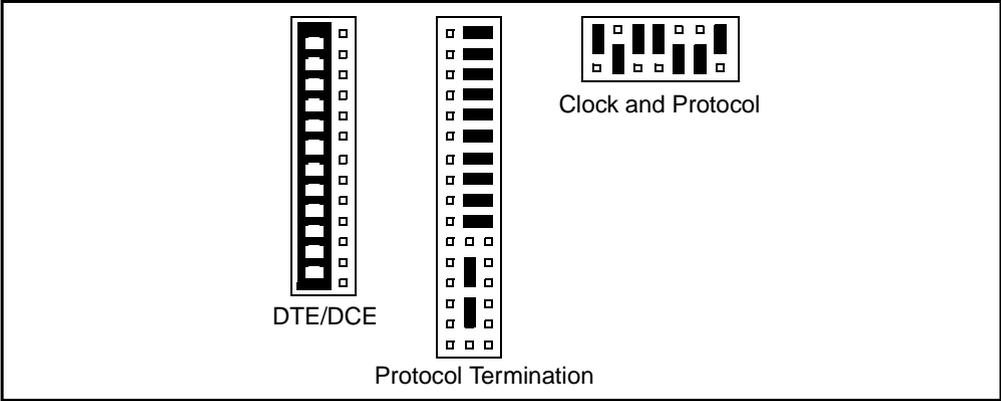
Transition Module Jumpers (DCE Type, EIA422 Protocol, DTE Clocking, DTE Transmit Data)
