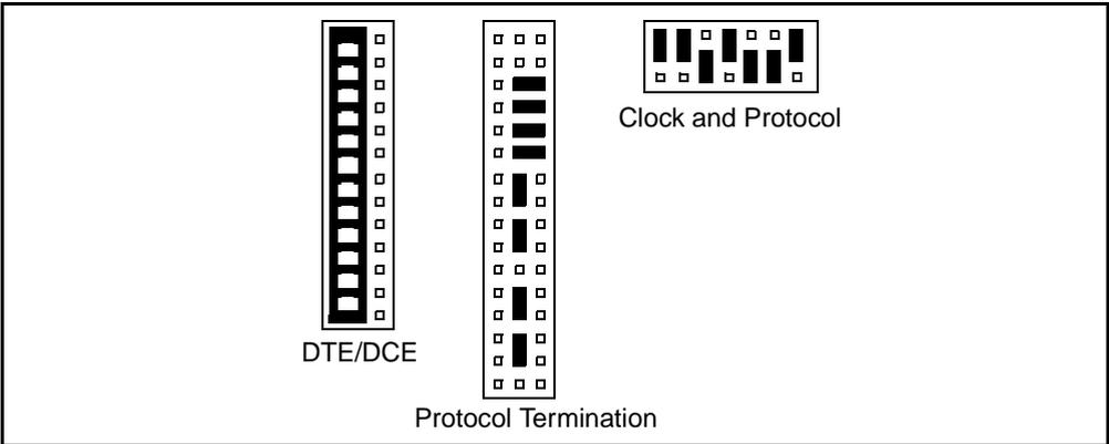
Transition Module Jumpers (DCE Type, EIA232 Protocol, DTE Clocking, DTE Transmit Data)
