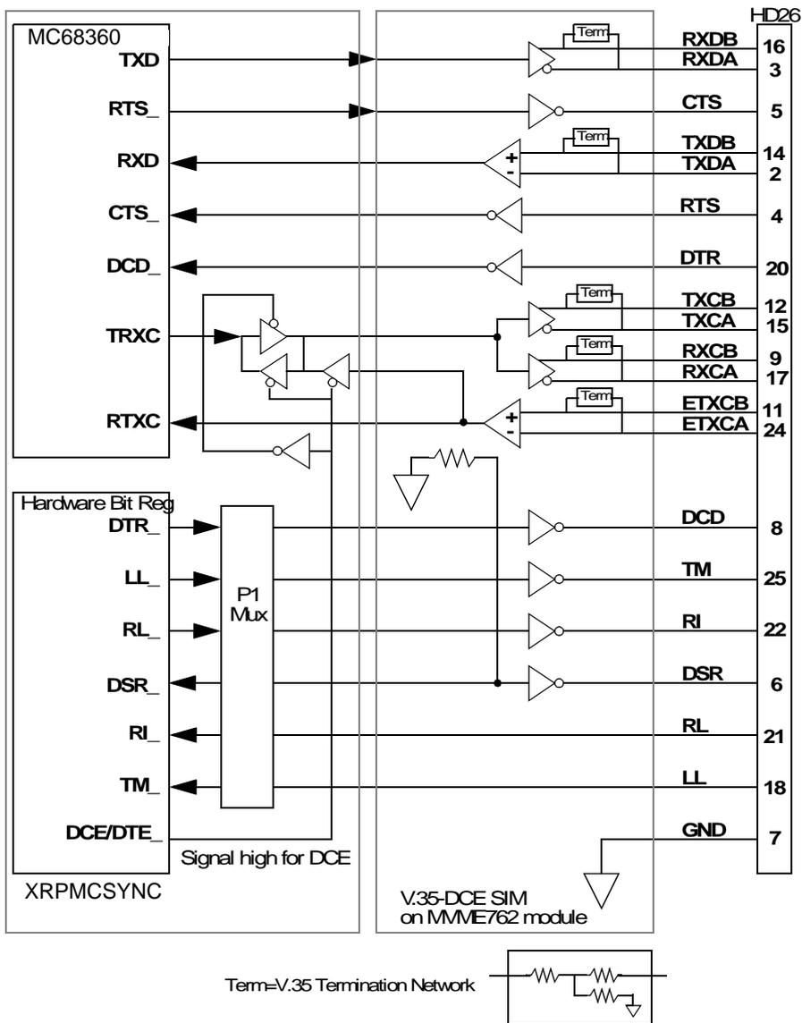
Figure 6-11. V.35-DCE Serial Port Configuration
