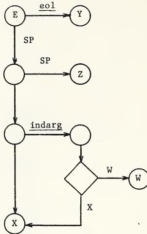
Note: The argument diagram is used to scan off the delimiter between the command word and its arguments (if any). It also handles indirection on the first argument of a command.
