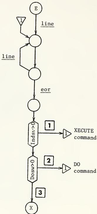
1. GET Argind, Forsw, Window position, and Present routine name from Stack. GET the indirect string off the Stack. Load routine if necessary. Link window to retrieved Window position
