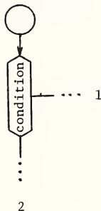
The logical value of "condition" is tested. If it is True, path 1 is taken. If it is False, path 2 is taken.
