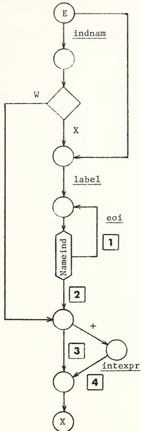
1. GET previous level's Nameind and Window position from the Stack. GET the indirect name off the Stack. Link window to retrieved Window position
