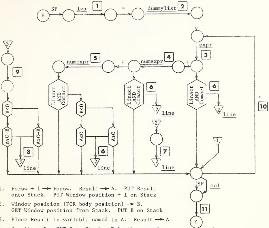
1. Forsw + 1 → Forsw. Result → A. PUT Result onto Stack. PUT Window position + 1 on Stack
