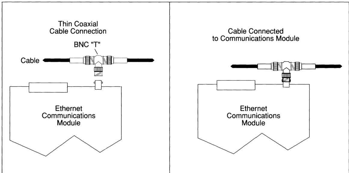
Figure 2-18. Thin Cable Ethernet Connection
