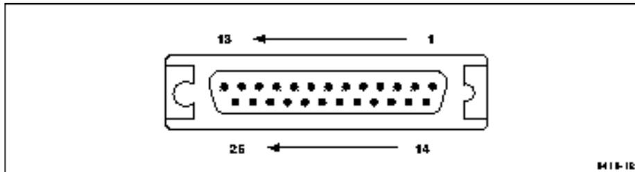
Figure A-4 Parallel Port Diagram.
