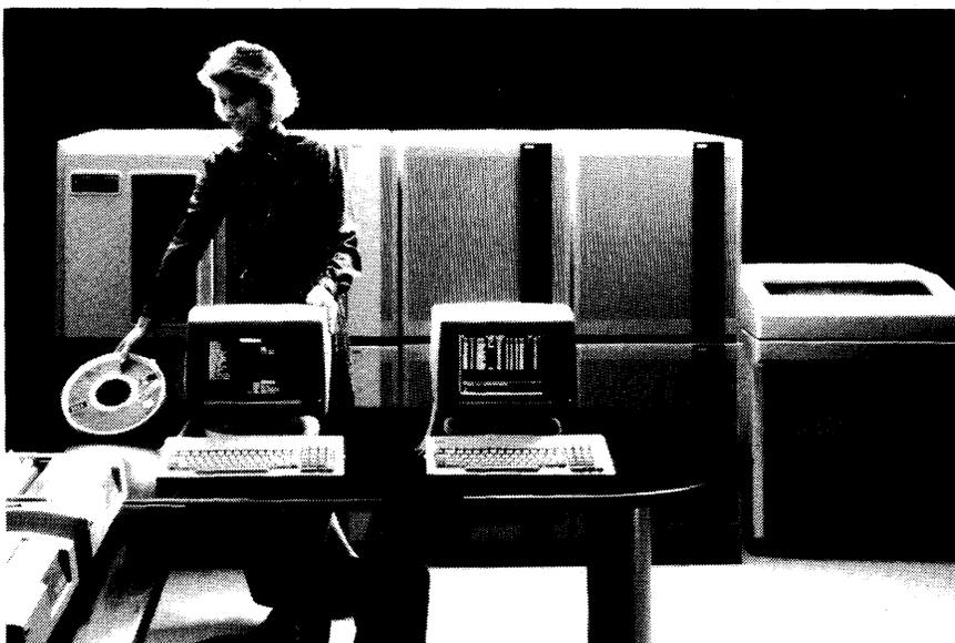
*The NCR 9800 is an on-line transaction processing system, based on multiple function-specific processors. The 9842 model is a mid-range configuration consisting of four application processors and two data storage processors. Each processor can contain up to 4 megabytes of memory.*
