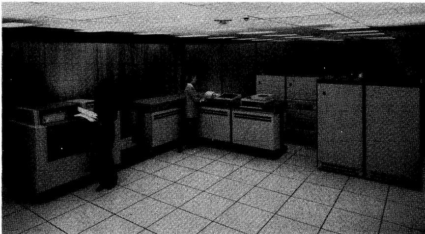
*The NCR Century 201, introduced in May 1974, provides raw processing power roughly equal to that of the original Century 200 but features expanded I/O capabilities for connection of larger and faster disc storage units. A basic 64K Century 201 system with 96 million bytes of disc storage can be rented for \$6,625 per month on a 1-year lease.*
