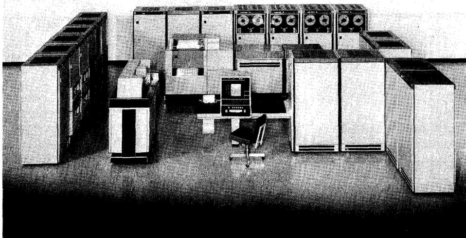
*With three times the internal performance of the Century 200, the 251 fits smartly athwart the sizeable gap between the 200 and the top-of-the-line Century 300. Shown here is a full-scale Century 251 installation with both disk and magnetic tape capability.*
