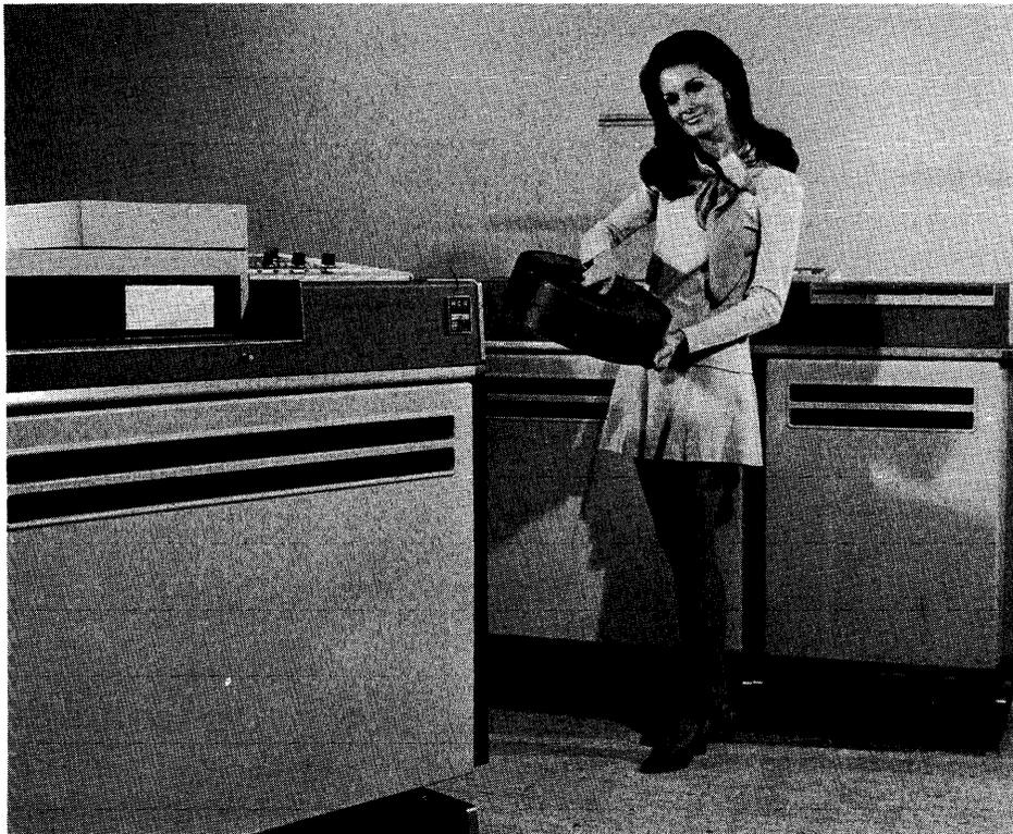
*The model holds one of NCR's 3-disc packs, which fits onto the dual-spindle disc unit behind her. The Century 50 processor, at left, includes an integrated 300-cpm card reader and control panel.*
