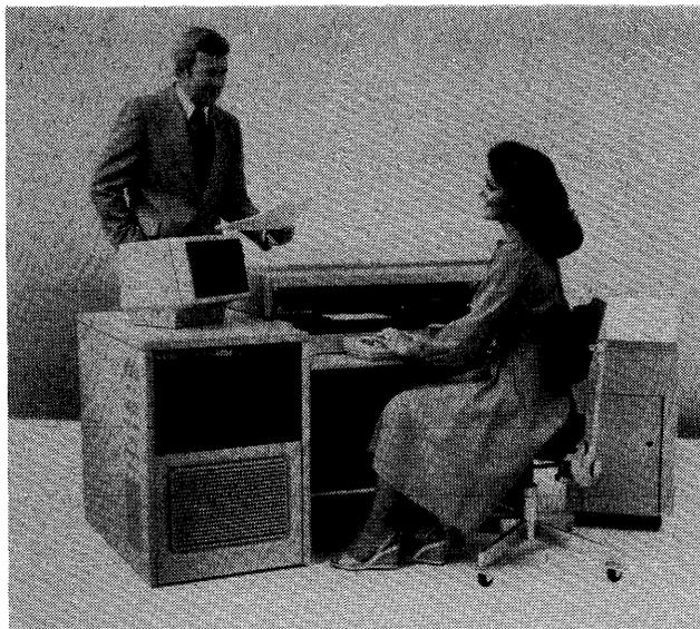
This NCR 8130 system includes a visual record printer that can accommodate continuous forms and journal rolls as well as cut forms such as ledger cards. Diskette storage capacity for the 8130 ranges between 900K bytes and 3.6 million bytes.
