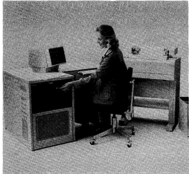
This NCR 8150 configuration consists of a CPU with 48K bytes of MOS memory, 4.9-megabyte cartridge disk drive, visual display terminal with 9-inch screen, keyboard, and serial matrix printer. The 8150 can be expanded to include up to 256K bytes of memory and 39.2 million bytes of disk storage.
