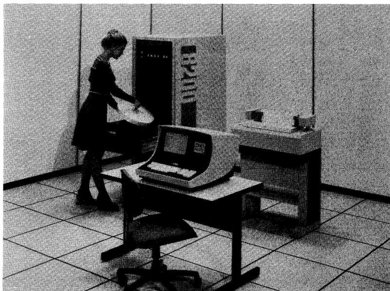
The NCR I-8231, the entry-level system in the 8200 Series, can support up to five terminals and accommodate NCR's complete library of interactive multiprogramming application programs. A basic I-8231 system includes a CPU with 64K bytes of memory, 9.8 megabytes of fixed/removable disk storage, a magnetic tape cassette system, and one CRT display terminal. This system can be purchased for \$22,245.
