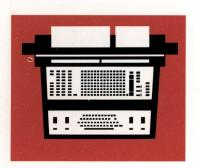
This brochure introduces the NCR 395 . . . a new, transistorized, electronic accounting and computing system. It is designed for varied data processing applications in all types and sizes of business.
