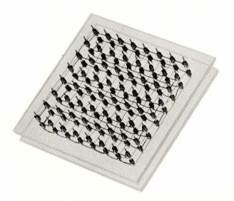
for storage of a bit. The Rod has been switched continuously at 5 megacycles at room temperature without adverse heating effects, and it can operate in either the word-ordered or the coincident-current mode from -100C to +200C.
