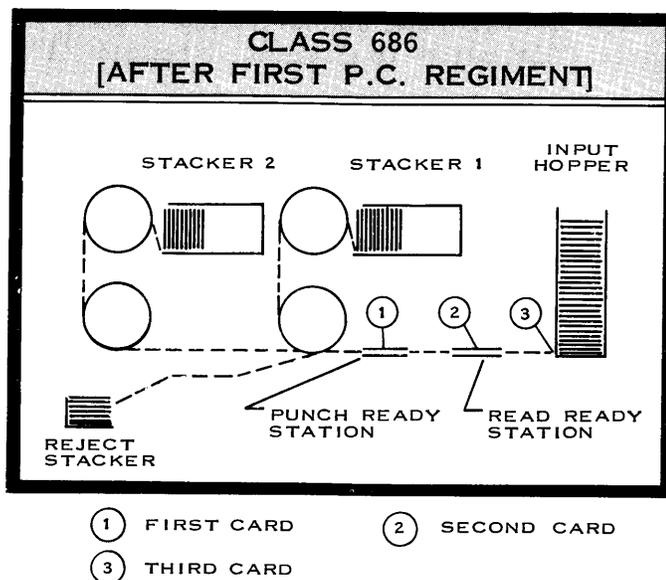
The first execution of the Card Regiment function moves the first card through the read station and makes the data from the first card available to the program. The first card stops in the punch ready station.
