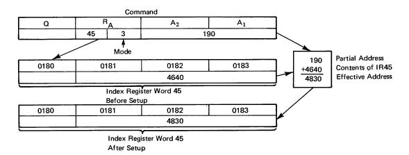
For added flexibility in addressing, all NCR Century series processors provide the ability for decremental indexing as well as incremental indexing. Decremental indexing, for example, may be used to search through a table in descending order.
