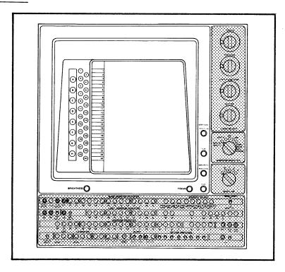
The CRT Display System is the main device used by the operator to communicate with the computer. With greater flexibility and rapid response, the CRT Display System provides the operator with instantaneous access to program and system status information.
