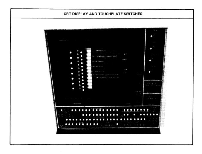
System software uses the CRT Display Unit to display the system status. The system status display is organized in an expanding, tree-like, hierarchical structure. The operator, by pressing the touchplate switches corresponding to the lines, may access any level of the tree-like structure. Information concerning peripheral availability, peripheral status, job queueing, or the list
