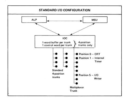
The standard I/O configuration may be expanded by adding two optional features. Each optional feature consists of adding two trunks to the standard I/O configuration, for a total of four or six 4-position trunks. Each optional trunk, like each standard trunk, has a "live" control word and a 1-word buffer. The NCR Century 251, with the standard I/O configuration, is capable of 10-way I/O simultaneity. The optional trunks increase the I/O capability to 12- or 14-way I/O simultaneity.
