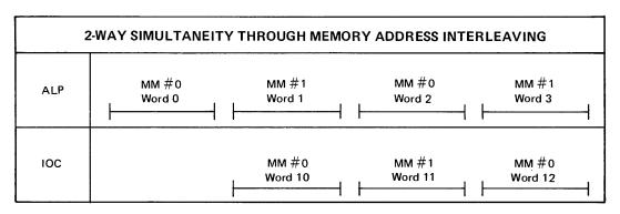
Memory locations are addressed by the least significant 18 bits of a 3-byte absolute address. The address bits are designated as L1 through L18. Of the 18 bits used, L3 through L18 constitute the word address, while L1 and L2 designate the byte within that word.
