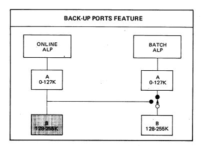
If memory unit B in the online system should become inoperative, one of the MSUs in the batch system can be switched to the online system manually. This keeps the online system "on the air" at full capacity. The batch processing system suffers some degradation because of the reduced memory storage, but it is still operational.
