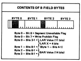
If the B address is not zero modulo four (0 mod 4), a PE results and the BAR/LAR registers remain undisturbed. If the processor is in the user state (S-flag OFF), the Command Code Trap is taken.
