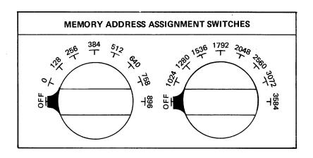
For example, assume that a 256K MSU is to be assigned to operate with addresses starting at 128K. Another MSU is to continue with sequential addresses where this MSU stops. The upper address range switch is placed in the OFF position; the lower address range switch is placed in the 128K position (starting address). The lower address range switch of the second MSU is placed in the 384K position, while the upper address range switch is in the OFF position.
