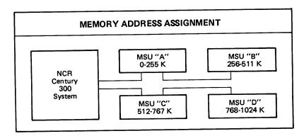
During the operation, memory unit C becomes inoperative. Since an MSU may be assigned to operate within any range of addresses, the unit with the highest address block, unit D, is reassigned to operate within the address range formerly assigned to unit C. Although some degradation results because of the reduced memory, the system remains operational. The inoperative unit is switched offline for testing and corrective action.
