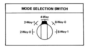
In 2-way-0 mode, the MSU functions with the first two memory modules interleaved in a 2-way mode and the second two memory modules functionally removed from the system. In 2-way-1 mode, the MSU functions with the second two memory modules interleaved in a 2-way mode and the first two memory modules functionally removed from the system.
