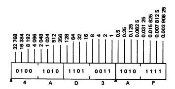
Each bit is examined and, if it is "true," its value is added to an accumulating total. This total is the decimal equivalent of the floating point representation. This step in the conversion process of the above number is illustrated below.
