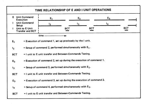
In the majority of cases, the operation of the E unit and the I unit is simultaneous during the running of the program. Exceptions are the indirect addressing, incremental indexing, or the sequential setup stages by the I unit. Before the I unit can complete these setup stages, the E unit must have terminated the execution phase of the previous command.
