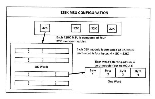
A maximum of 8 MSUs may be connected to the processing units, so the maximum memory capacity needed for the system determines the individual capacity of each MSU. Because of the limitation of eight maximum MSUs in a system, within the range of sizes shown in the following table, the MSUs may be only in certain increments.
