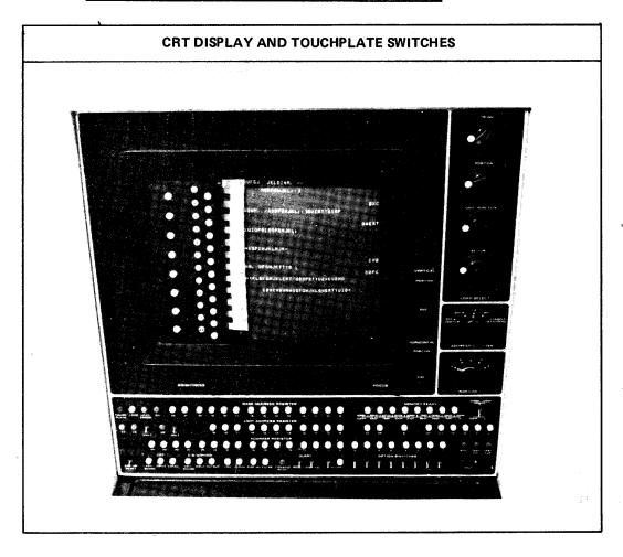
System software uses the CRT Display Unit to display the system status. The system status display is organized in an expanding, tree-like, hierarchical structure. The operator, by pressing the touchplate switches corresponding to the lines, may access any level of the tree-like structure. Information concerning peripheral availability, peripheral status, job queueing, or the list of pending messages is immediately available to the operator, as shown on the following illustration.
