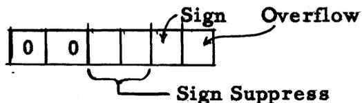
The sign digits may be interpreted binary digit by binary digit the same as the binary sign digits (See Section II, page 4). The decimal code is represented outside the machine according to the following table:
