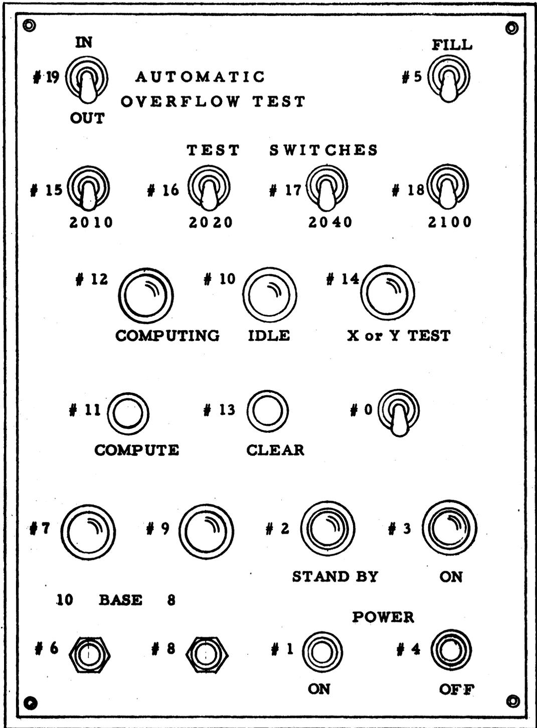
**Figure I. Computer Control Panel**
