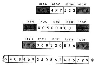
• First LOAD the Accumulator with the contents of the 2-slab word starting at location 02 345. The Accumulator now contains:
