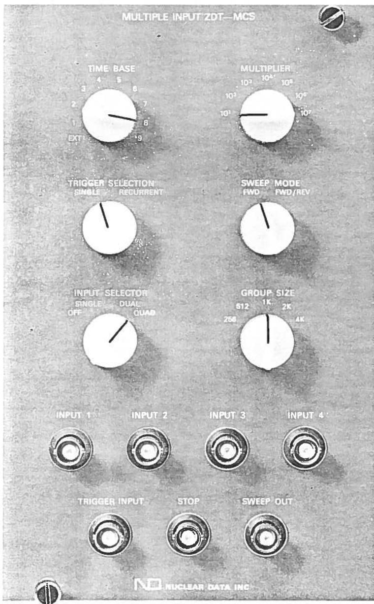
**INPUT SELECTOR** - Four position rotary switch selects number of inputs. OFF, SINGLE, DUAL and QUAD positions. (If the module is not being used, switch should be in OFF position.)
