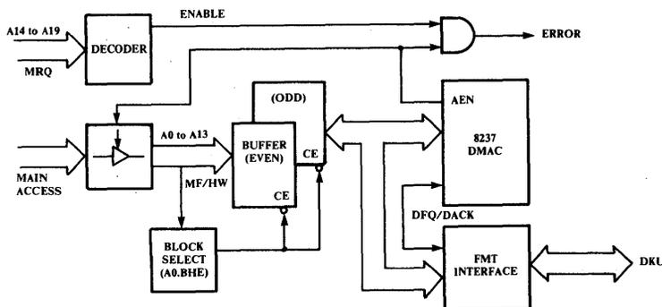
Figure 2-2 Buffer Control Block
