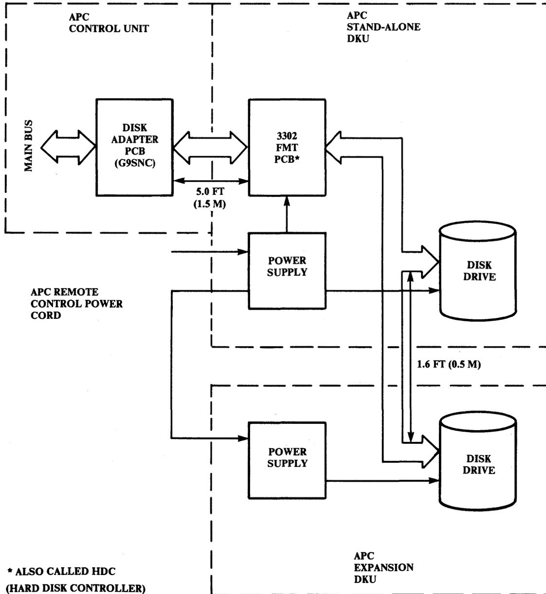
Figure 1-3 APC Stand-Alone/Expansion DKU Functional Block Diagram
