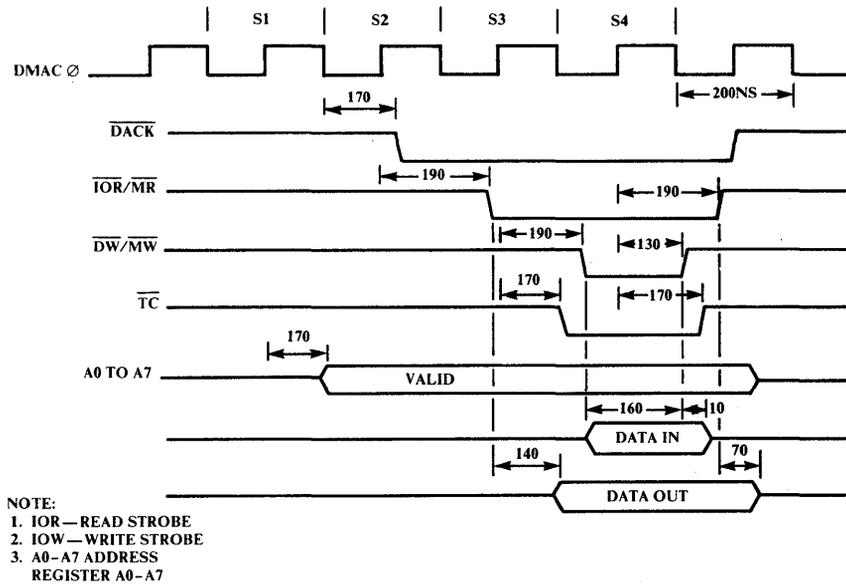
Figure 2-6 DMA Access Timing
