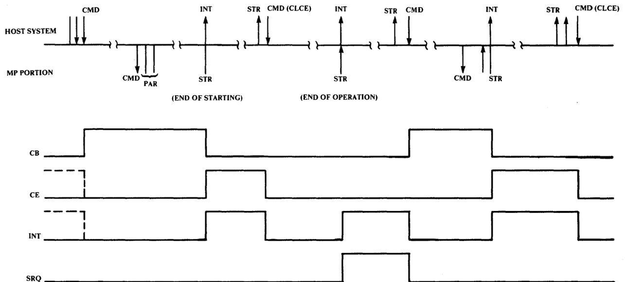
Figure 2-15 Seek/Recalibrate Timing
