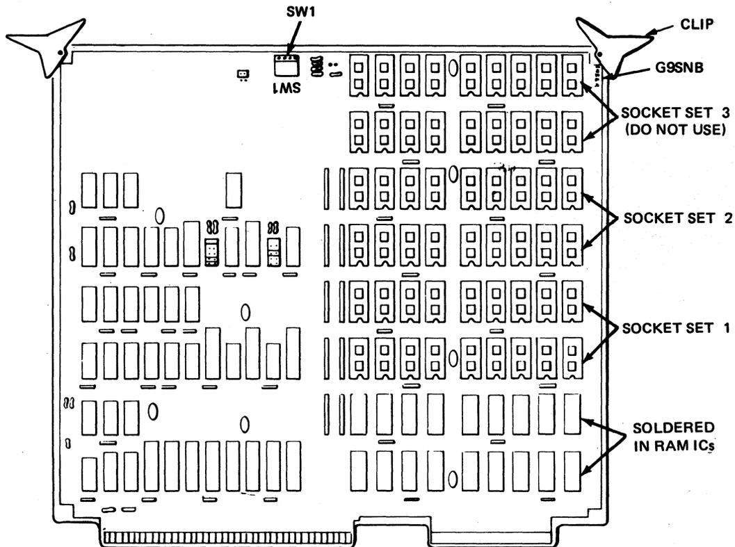
**Figure 4 The APC-H31 Memory Expansion Unit PCB (G9SNB)**
