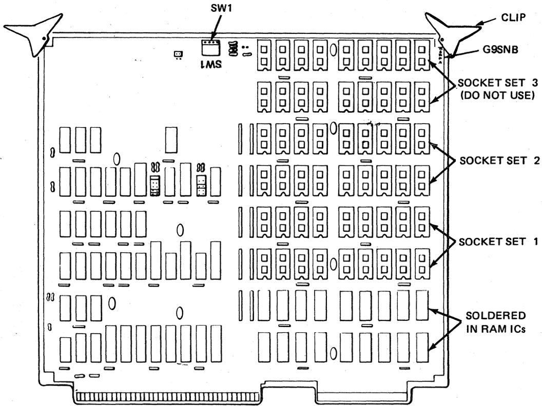
**Figure 1. The APC-H31 Memory Expansion Unit PCB (G9SNB)**
