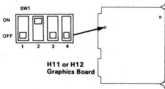
SWITCH SETTINGS FOR THE APC-H11 OR H-12 WHEN THE APC DOES NOT CONTAIN AN H-08 EXPANSION MEMORY BOARD (G9PTV).
