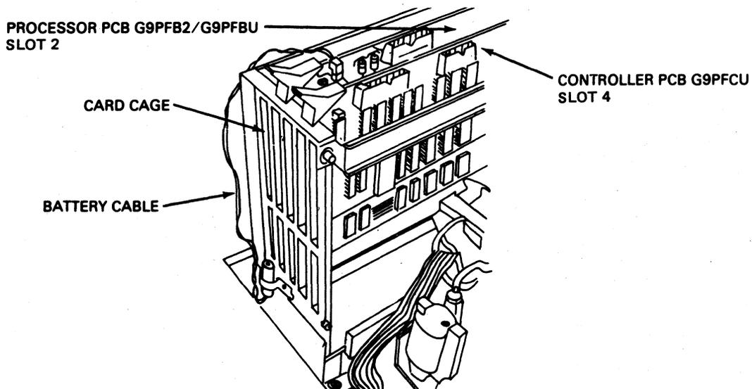
**Figure 11 Card Cage (Front View)**
