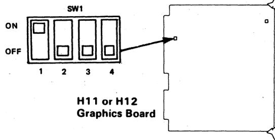
**Figure 8 Switch Positions for the APC-H11/H12**
