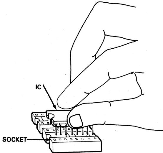
**Figure 5 Inserting the IC into the Socket**
