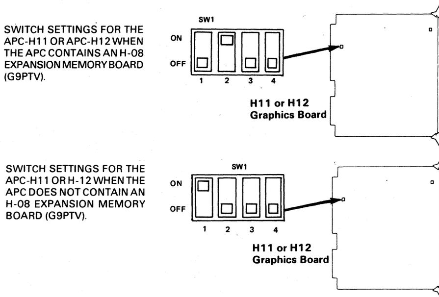
**Figure 9 Switch Positions for the APC-H11/H12**
