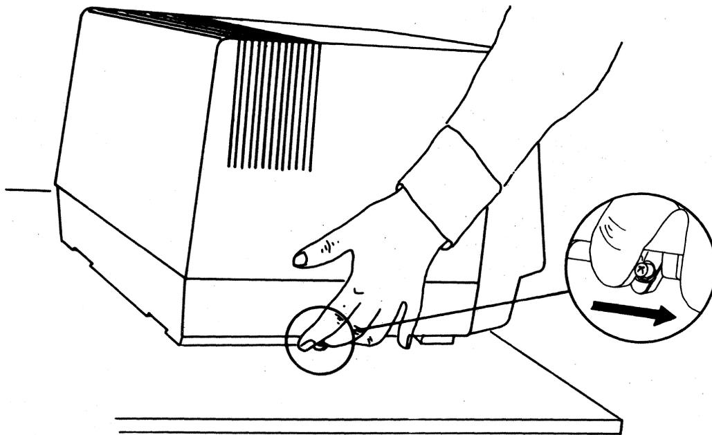
Figure 10 Removing the APC Top Cover
