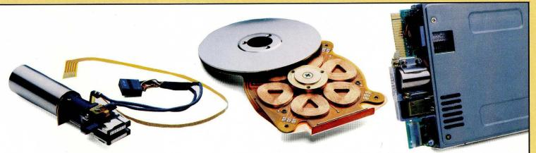
Positioner and Head Assembly — OKIDATA's head assembly has an integrated compact linear stepping motor, and is engineered with only one moving part, eliminating such mechanical assemblies as bands and lead screws.
