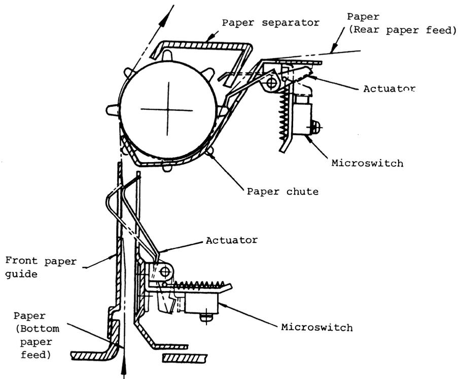
Fig. 5-6 Paper Out Detecting Mechanism
