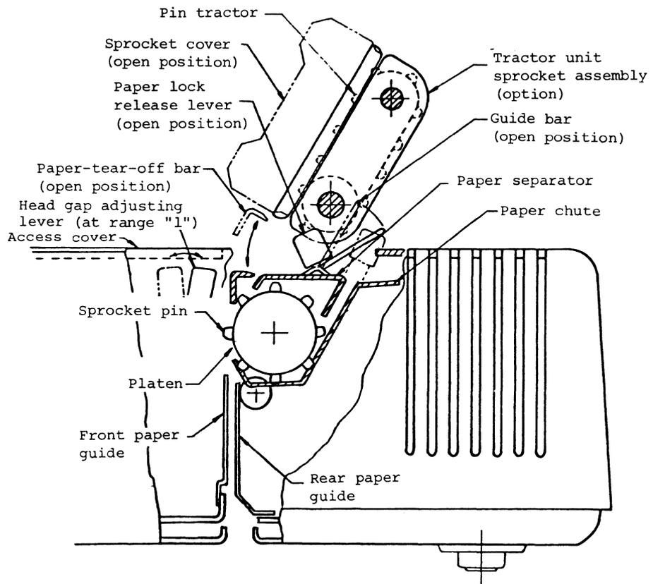
Fig. 3-7 Sprocket Paper Loading Method
