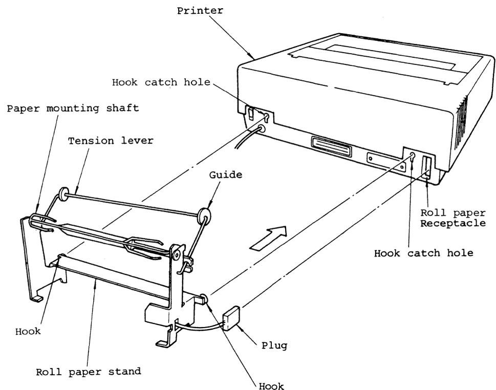
Fig. 3-5 Roll Paper Stand Mounting Method
