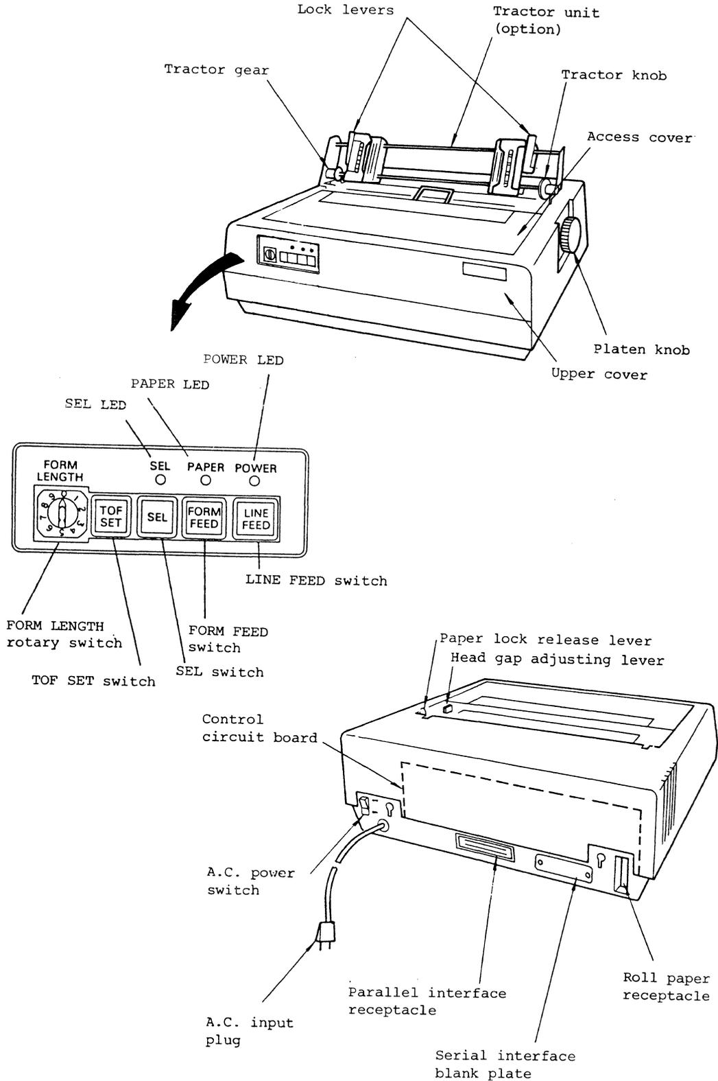
Fig. 3-3 Operating Controls, LEDs and Others
