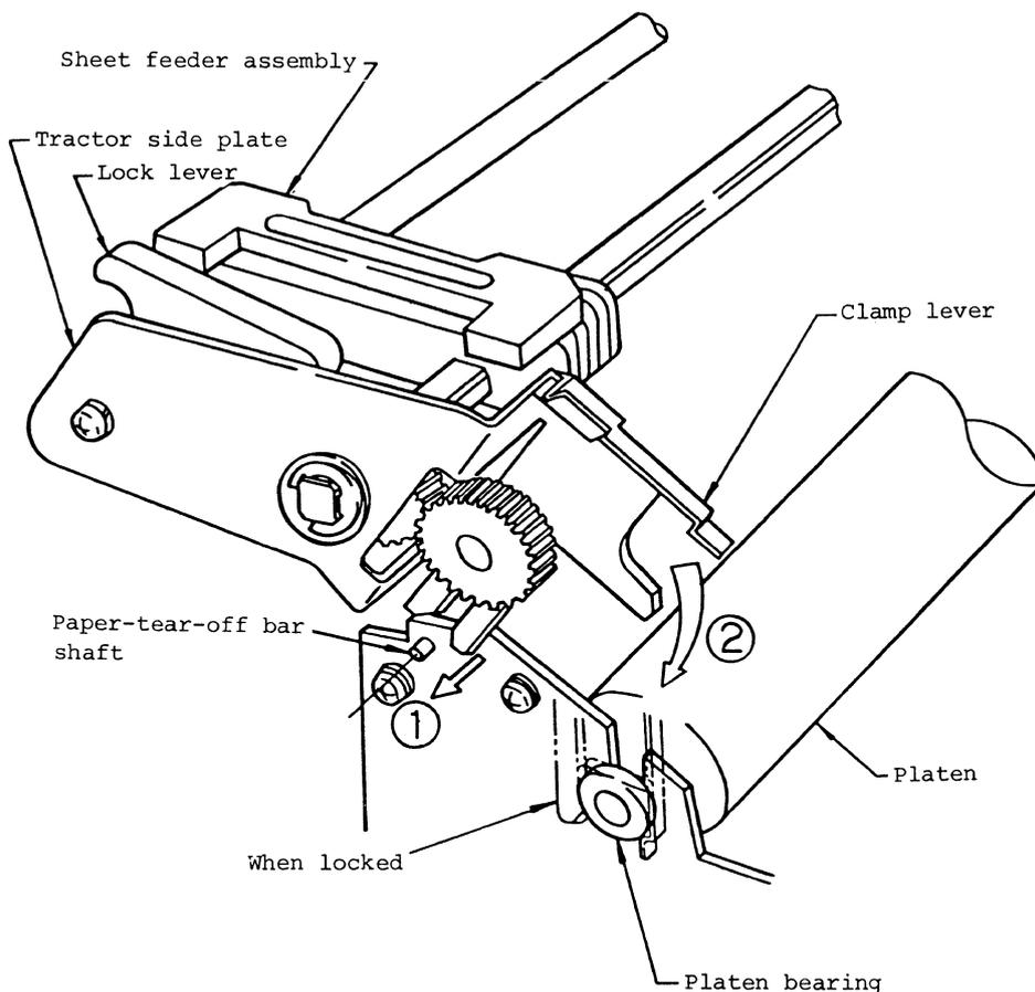
Fig. 3-4 Tractor Unit Mounting Method
