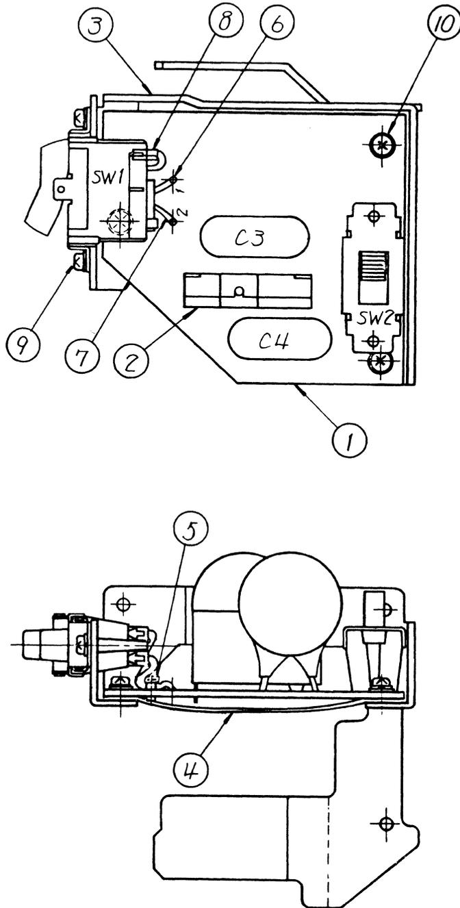
Fig. 8-12 LEPW-2 Circuit Board Assembly (3LX-86727-2) (for 220/240 V)
