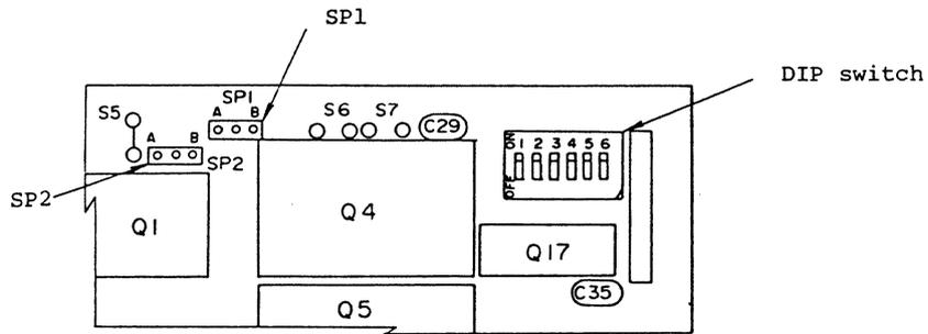
Fig. 4-3 DIP Switches and Jumper Plugs on Control Circuit Board
