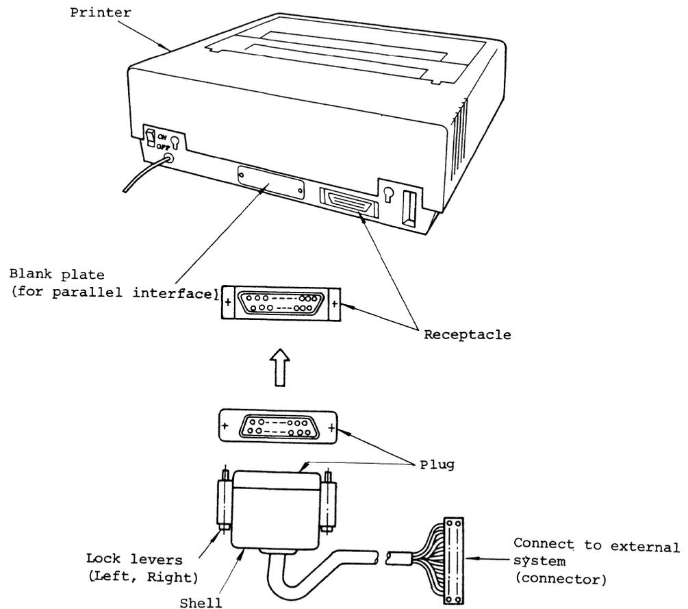
Fig. 3-2 Low Speed Serial Interface Connection Diagram
