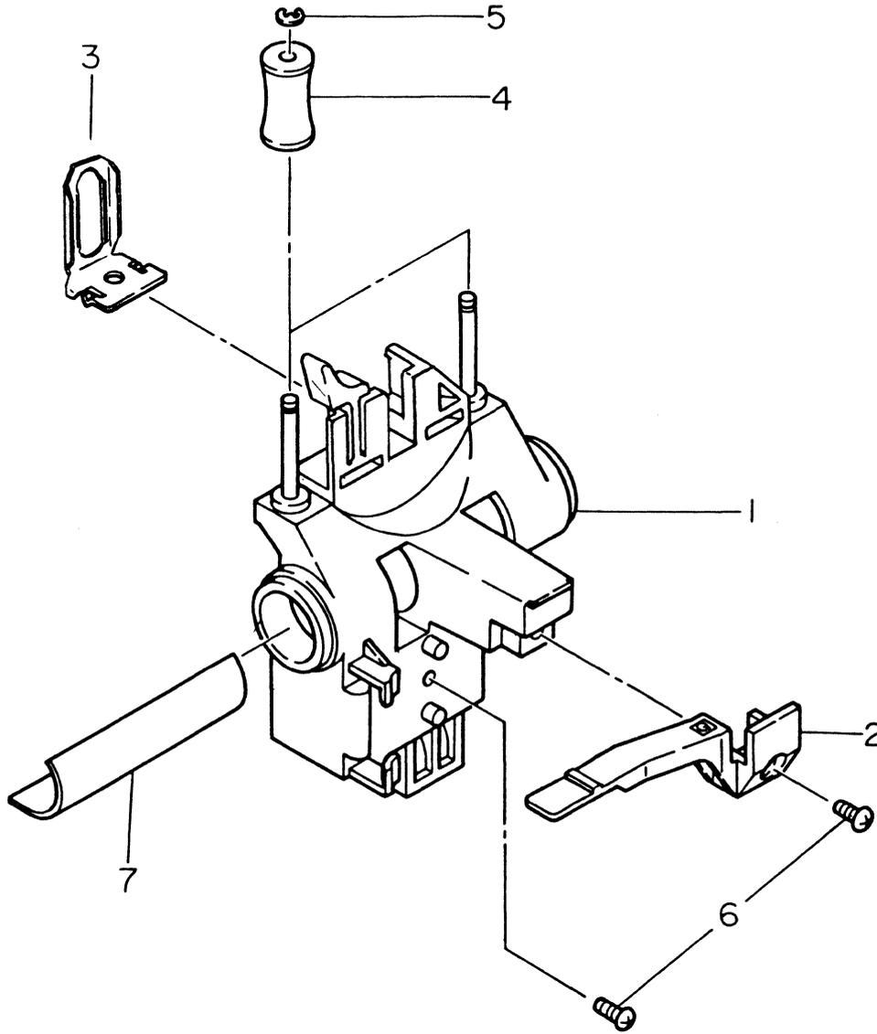
Fig. 8-7 Carriage Assembly (4LR-191870)
