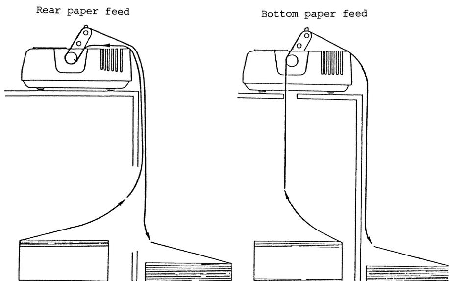
Fig. 3-8 Sprocket Paper Positioning
