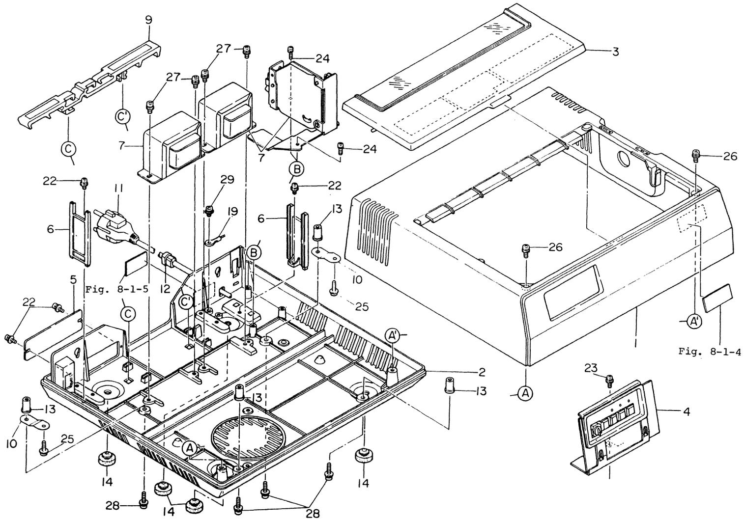
Fig. 8-8 Cover Unit (1LM-61521-3) (for 220/240 V)
