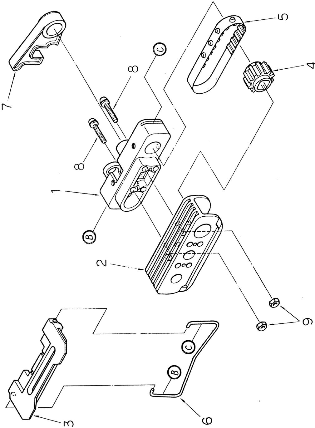
Fig. 8-15 Sprocket Assembly (R) (FMX-35100-2)
