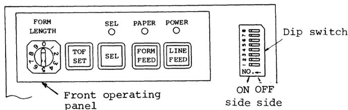
Fig. 4-2 DIP Switches on Operation Panel Circuit Board
