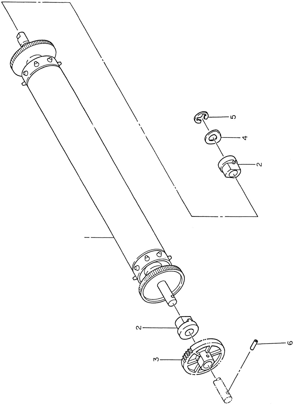
Fig. 8-4 Platen Assembly (3LR-129900-3)
