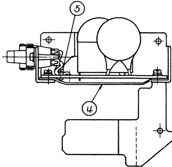
Fig. 8-12 LEPW-1 Circuit Board Assembly (3LX-86727-1) (for 115 V)
