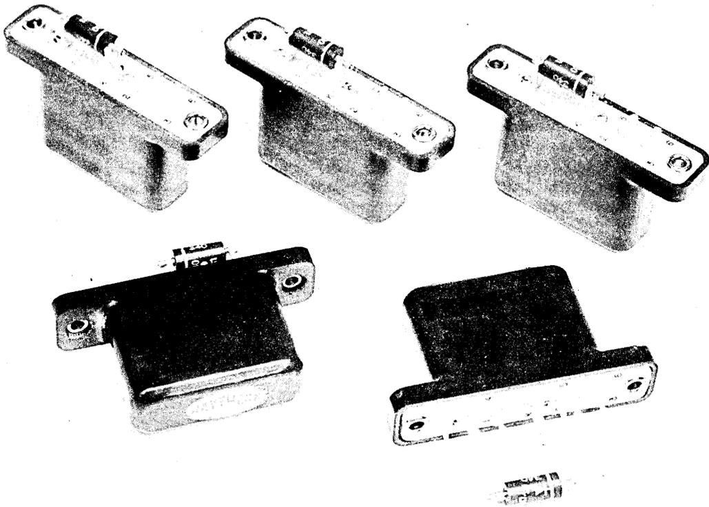
Figure 2. Raytheon magnetic shift register SR-100.
