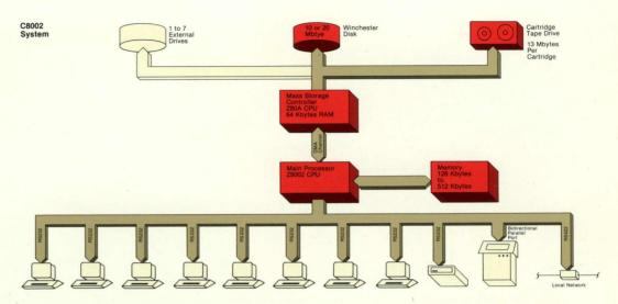
The C8002's advanced system architecture, integrated mass storage peripherals and unique packaging result in exceptional cost effectiveness. The entire system consists of six basic modules:
