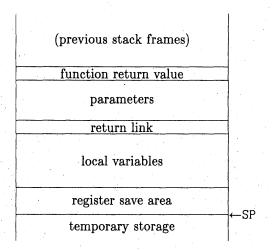
Not all of the fields will be used by the compiler for every procedure; only the return link is present in every frame. It is the responsibility of the called procedure to remove the parameters and local variables from the stack before a return is made to the caller.
