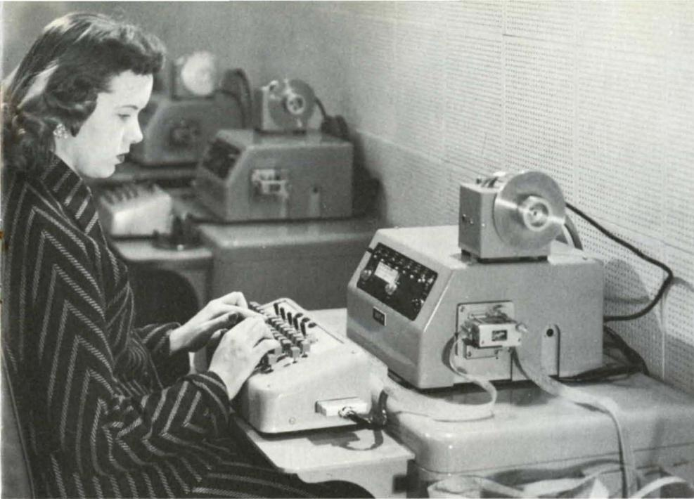
Instructions and input numbers for the Oracle must be punched in coded form on paper tape.
