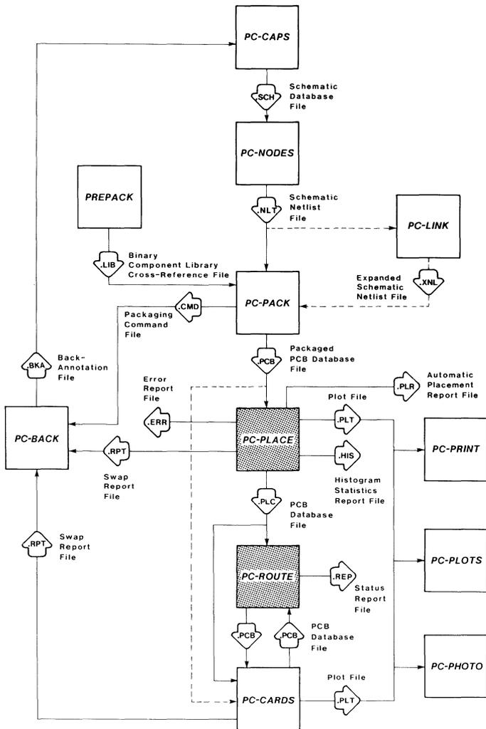
Figure 1. End-to-End PCB Design Flow Using PC-PLACE and PC-ROUTE
