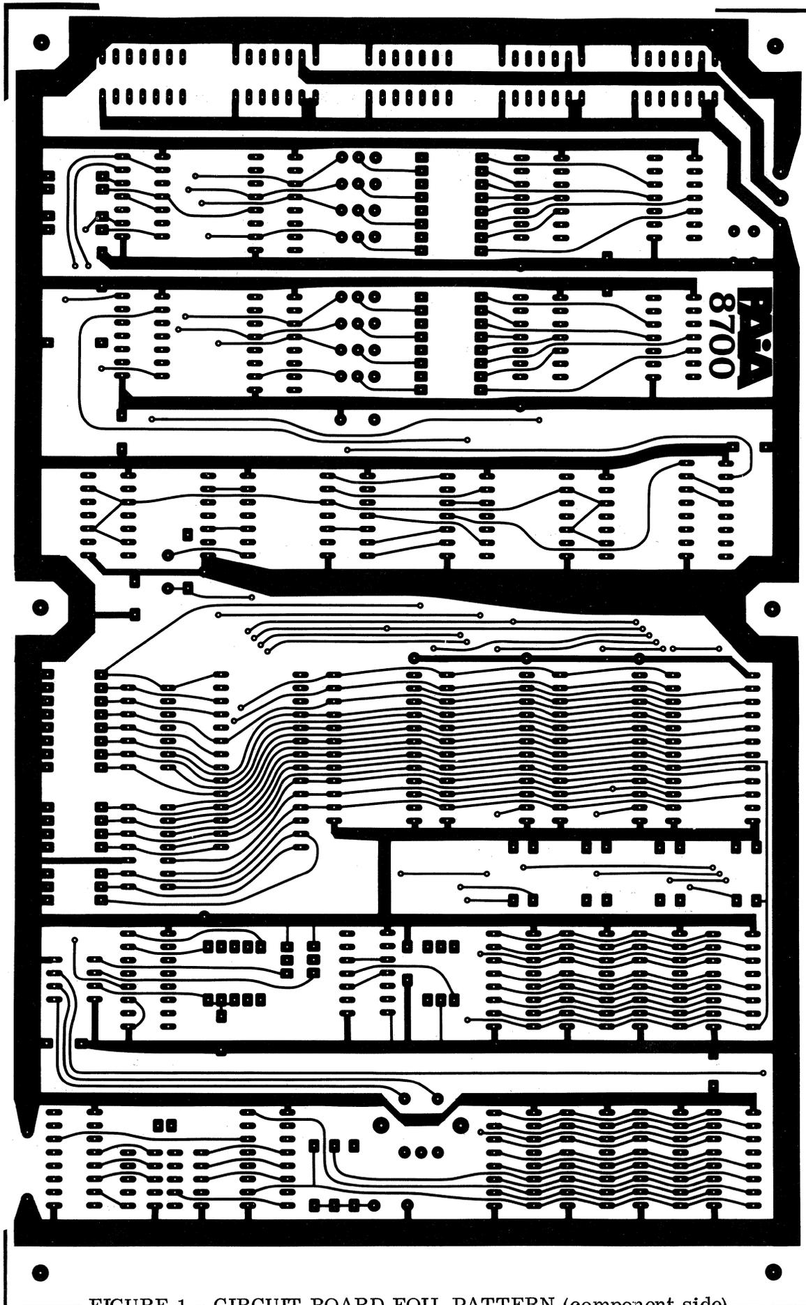
FIGURE 1 - CIRCUIT BOARD FOIL PATTERN (component side)
