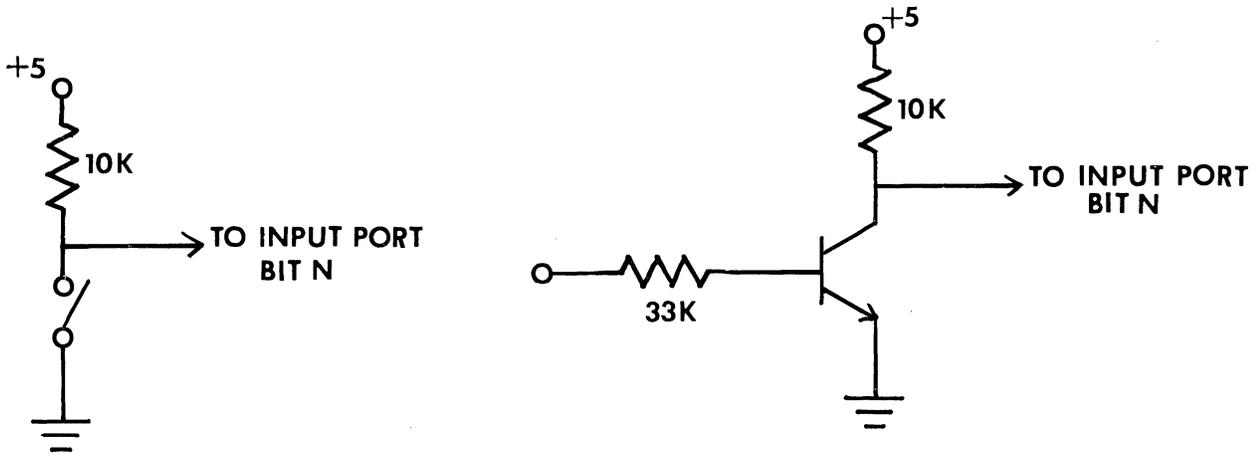
and note that if the transistor or switch above is "on", it represents a 0 input to that pin of the port.
