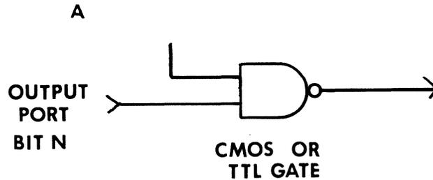
Because of the static nature of these outputs, practically any number of CMOS gates can be driven. (The limiting factor is the risetime of the output as the additional capacitors that the inputs of the gates represent are added.) If you like, and if the specifications of the power supply are not exceeded, power for the peripheral device can be picked up on J2 as are the signal leads.
