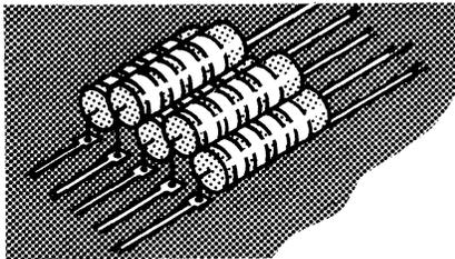
Using parts placement designators and the parts placement drawing in figure 3 as guides, solder the following resistors in place. Notice that many of these resistors are close together and consequently may need to be "stacked" as shown to the left.
