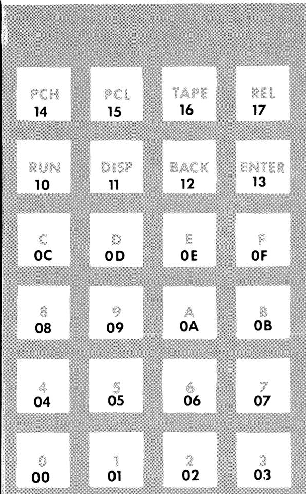
The keyboard is used by the monitor for control of user data and program entry as well as operation of the PIEBUG debugging tools, but may also be read by the user's programs employing a variety of techniques.
