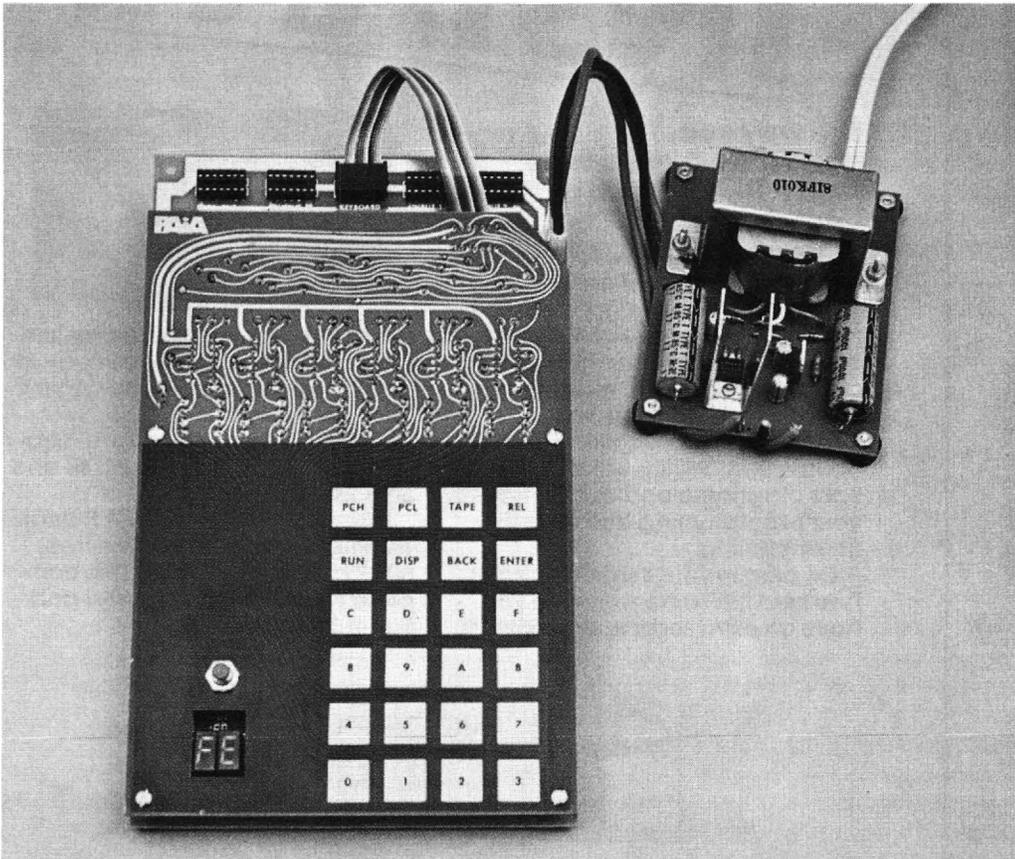
*Photo 1. The PAIA 8700 and its optional power supply. The keyboard is mounted on top of the CPU board with 3/4 inch standoffs. The vacant IC sockets at the top are the input/output connectors. The expansion connectors are under the keyboard. Note the reset button and digital readout in the lower left-hand corner.*
