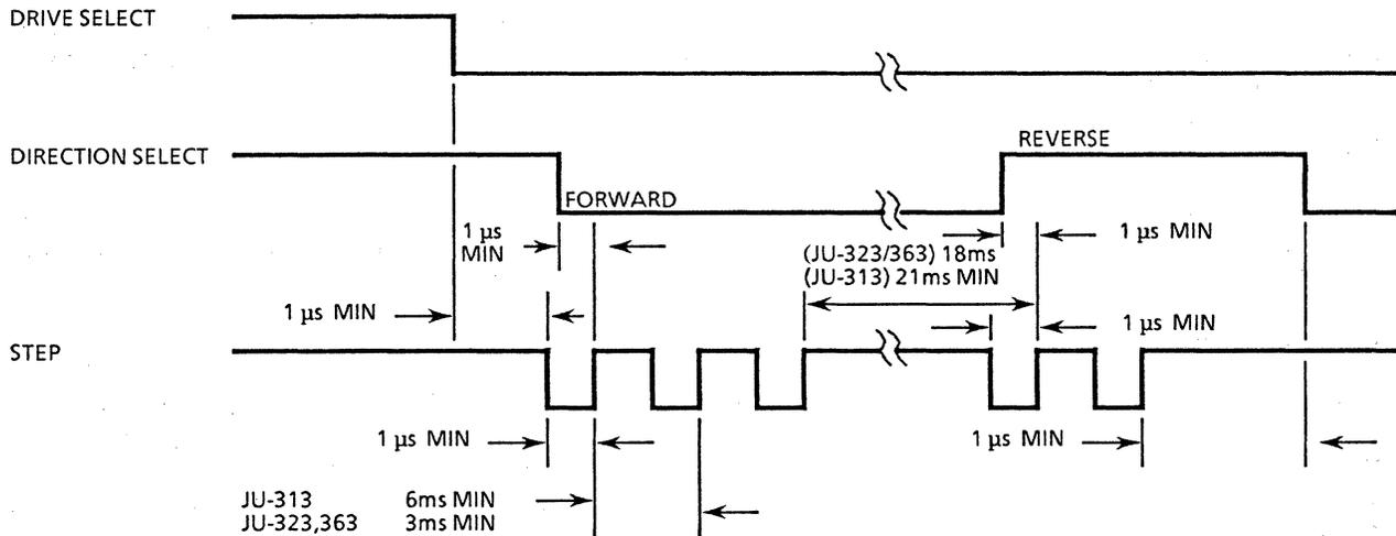
FIGURE 1-3 TRACK ACCESS TIMING
