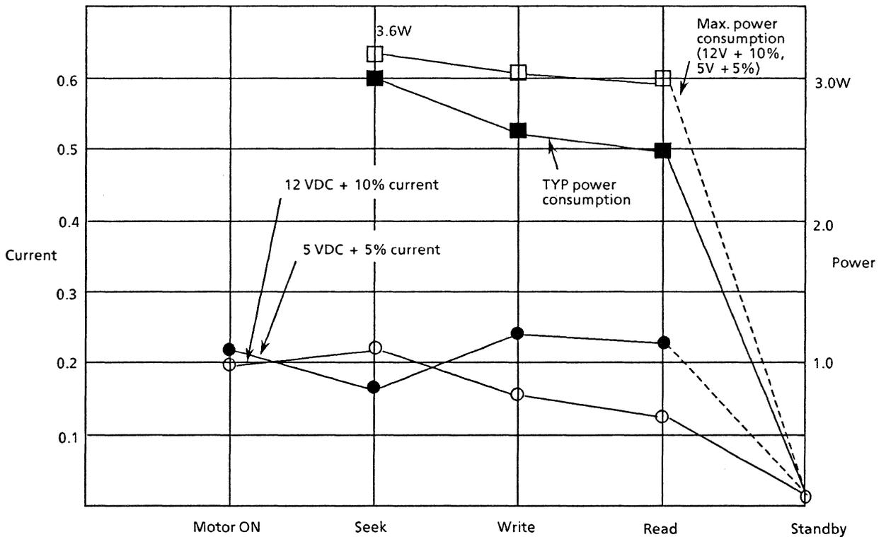
FIGURE 1-1 CALCULATION METHOD OF POWER CONSUMPTION
