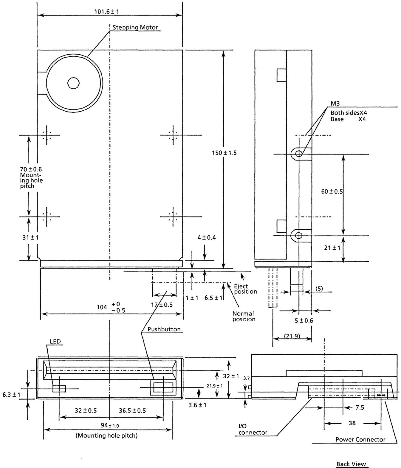
FIGURE 4-2. MECHANICAL DIMENSIONS
