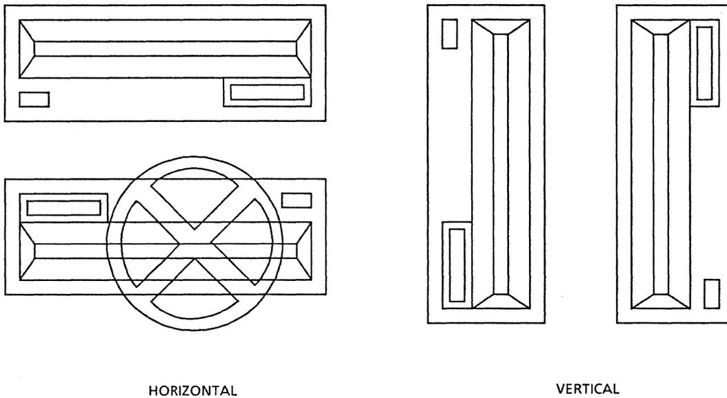
FIGURE 4-1. RECOMMENDED MOUNTING POSITIONS
