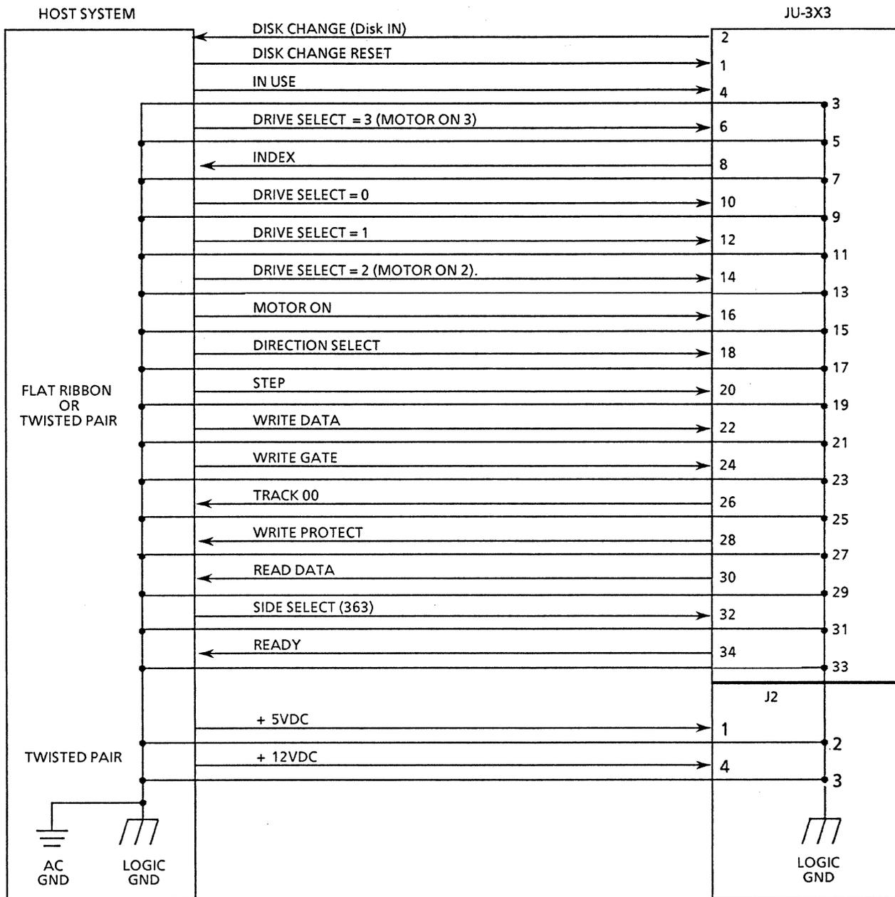
FIGURE 2-1 INTERFACE CONNECTIONS
