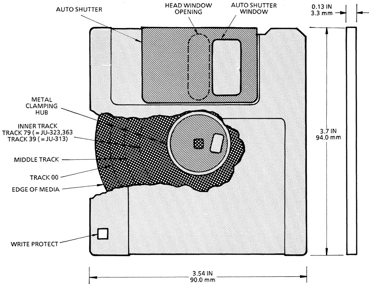
FIGURE 8-2 MICROCARTRIDGE NOMENCLATURE
