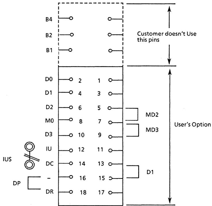
FIGURE 7-2 SHORTING BAR P2 PIN ASSIGNMENT
