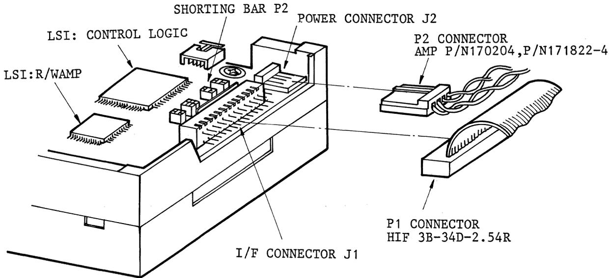
FIGURE 3-1 INTERFACE CONNECTORS LOCATIONS
