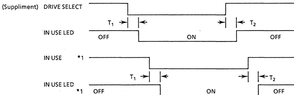
\*1) PIN11 & 12 (Pin Post P2 on PCB).
