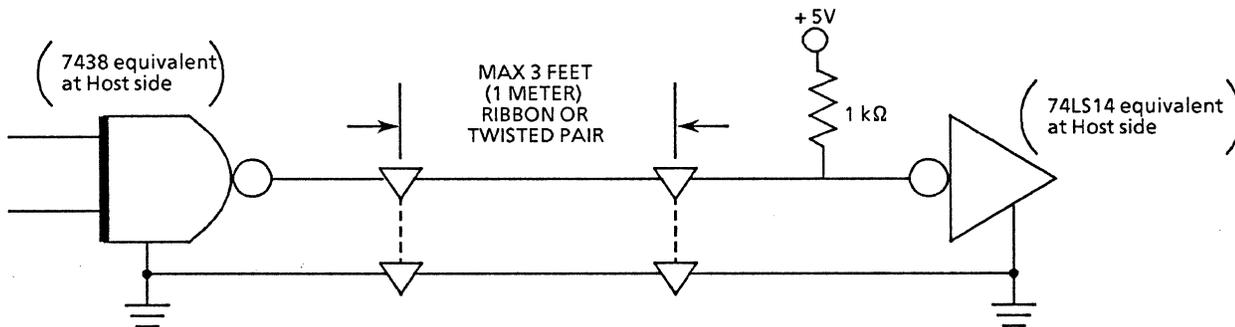
FIGURE 2-2 INTERFACE SIGNAL DRIVER/RECEIVER
