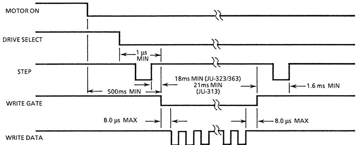
FIGURE 1-8 WRITE INITIATE TIMING
