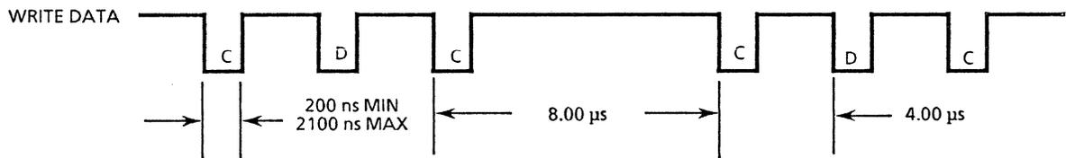
FIGURE 1-9 WRITE DATA TIMING (FM)
