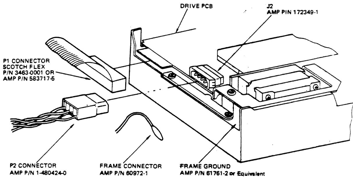
FIGURE 6-1 INTERFACE CONNECTORS LOCATIONS
