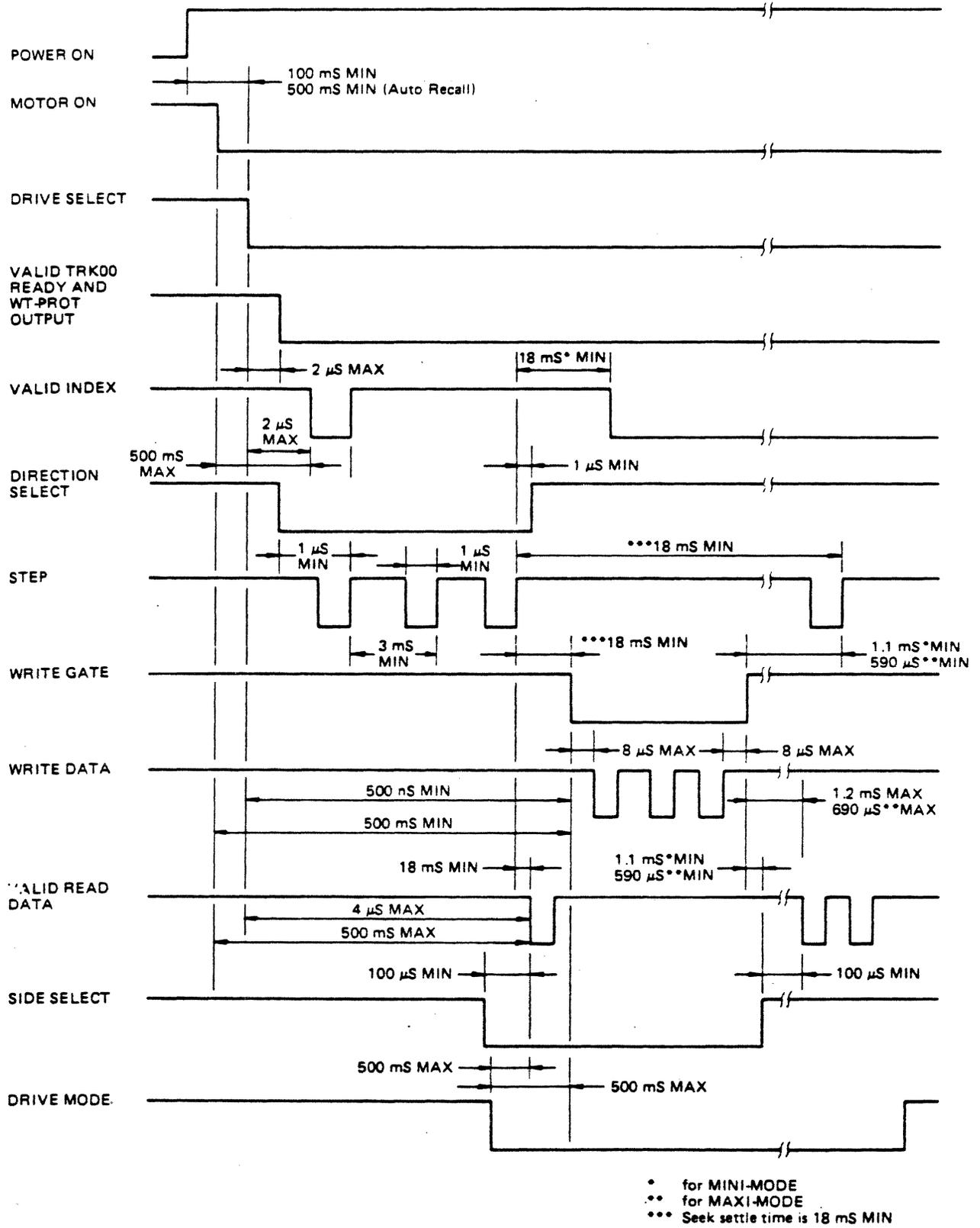
FIGURE 5-6 GENERAL CONTROL AND DATA TIMING
