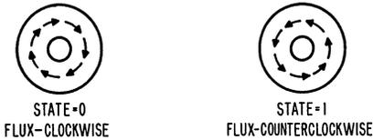
Fig. 5-1. Magnetic cores are used as memory stores.
