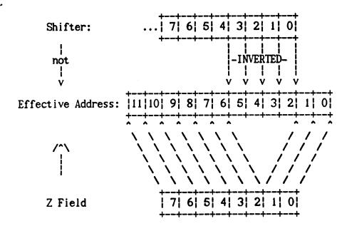
The Z field is derived from the target by the microassembler (see section 3.4.3 for details).
