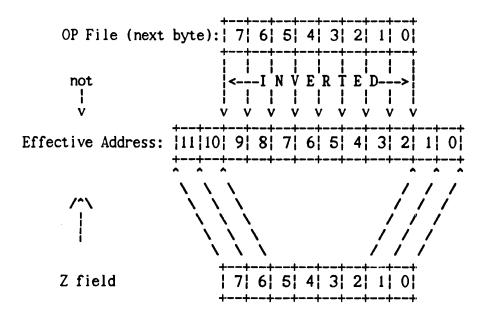
If the Op file is empty (BPC[3] = 1) then the OP File bits are forced to #377. Since these bits are inverted in the effective address, control passes to the base address generated from the Z bits (effective address bits 9..2 are zero). It is necessary to place a special refill function at this address ('Zaddr') which fetches four new bytes, increments UPC by four, performs a LOADOP (see section 3.5.1.4), and repeats the NEXTINST. The return from this special refill should be via NextInst.
