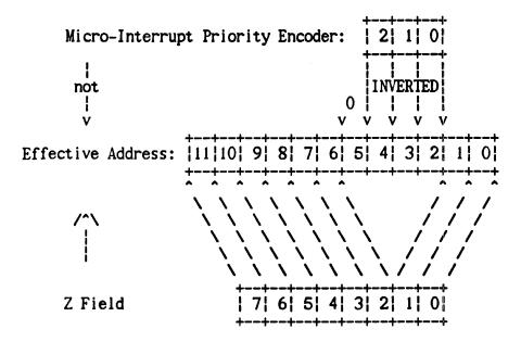
The microassembler derives the Z field from the target (see section 3.4.3).
